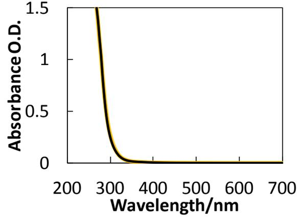
**Figure S5.** UV-Visible absorption spectra for an as-synthesized blue-plasma sputtered sample (black curve), and the same sample after 3 days (orange curve).
