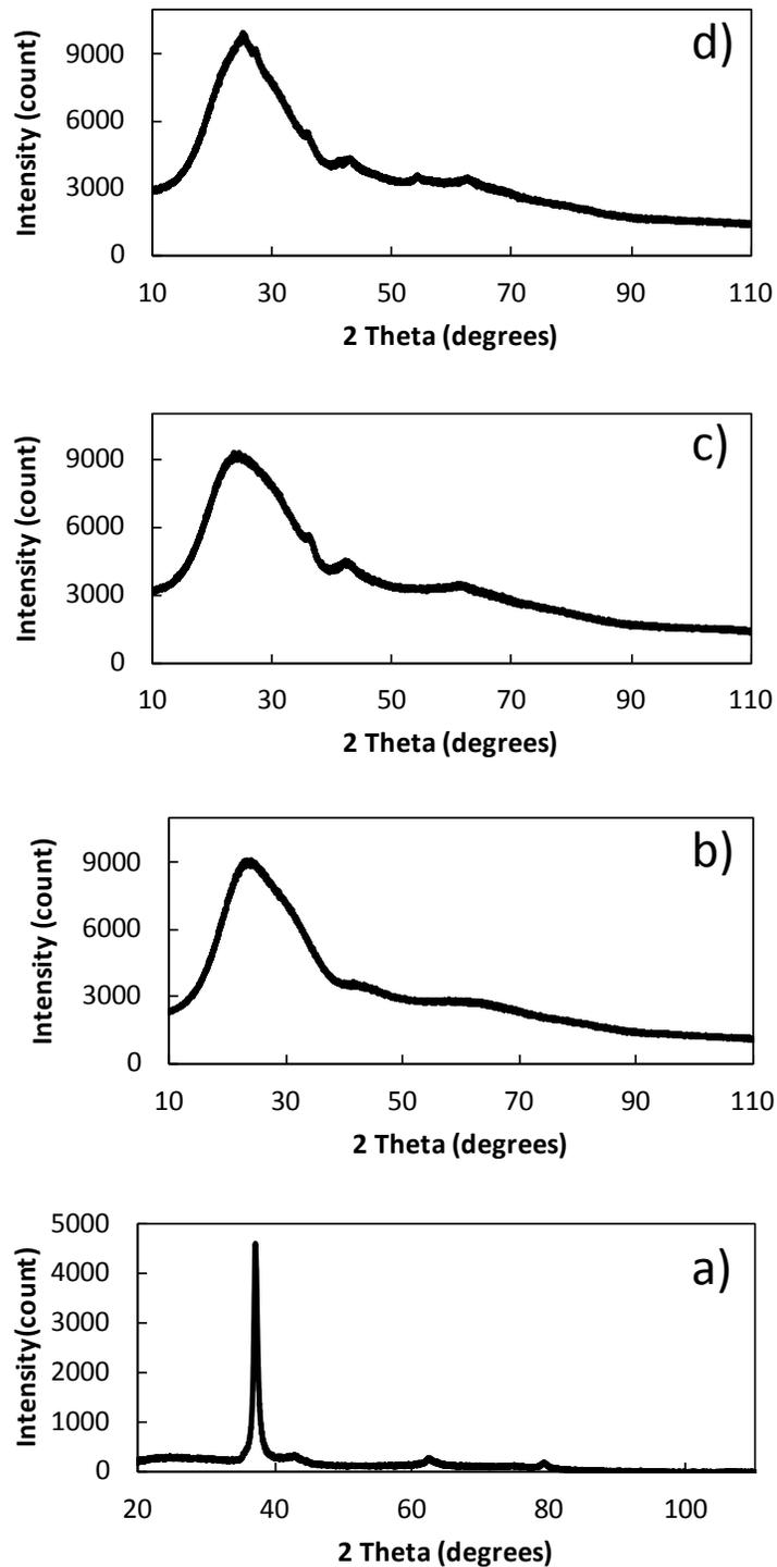
**Figure S2.** XRD patterns of samples obtained via (a) green-plasma sputtering; (b) glass substrate without sputtering Ti on it; (c) blue-plasma sputtering; (d) corresponds to sample (c) after annealing at 500 °C for 2 h under N<sub>2</sub>.
