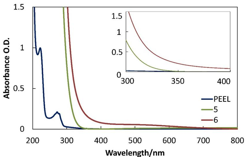
**Figure S3.** UV-Vis spectra of PEEL, and the 30 minutes blue-plasma sputtered samples that underwent to also 30 and 60 minutes of green-plasma sputtering for sample 5 and 6 (also see Table 1 in the main text), respectively.
