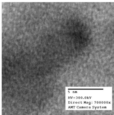
**Figure S4.** TEM image taken from a sample sputtered in blue-plasma condition for 30 minutes at 400 mA.
