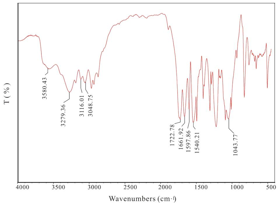
**Fig. S7** IR spectrum of chitosan bis(4-chlorophenylcarbamate)-(isobutyrylamide) (P1)
