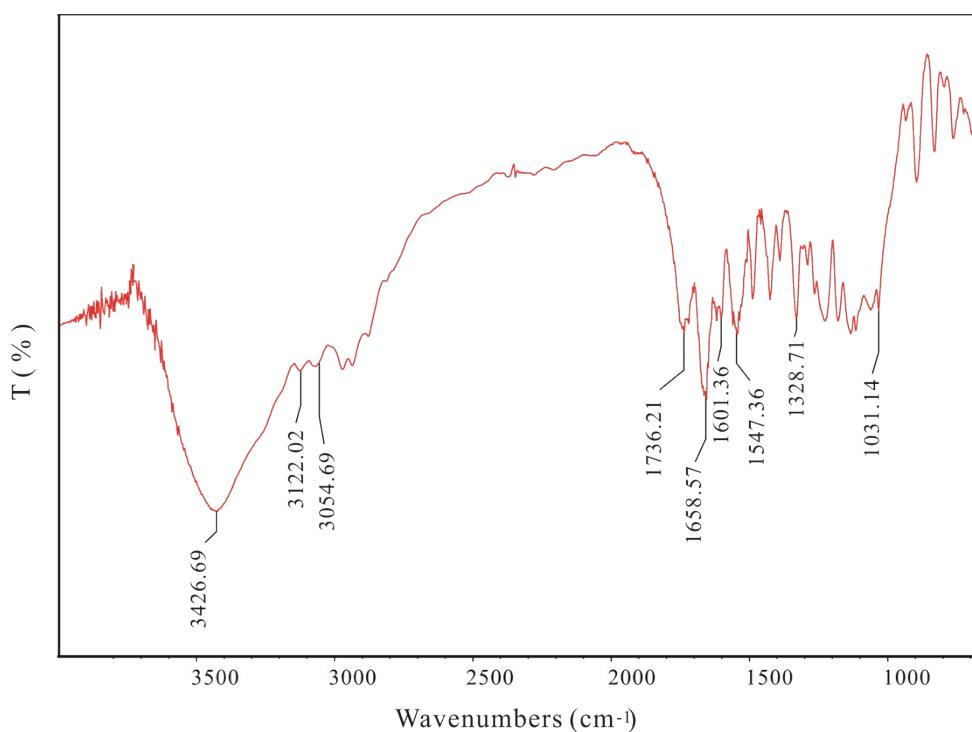
**Fig. S10** IR spectrum of chitosan bis(4-chloro-3-trifluoromethylphenylcarbamate)-(isobutyrylamide) (P4)
