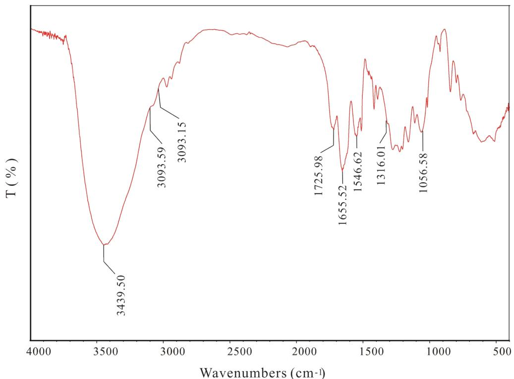
**Fig. S12** IR spectrum of chitosan bis(4-trifluoromethoxyphenylcarbamate)-(isobutyrylamide) (P6)
