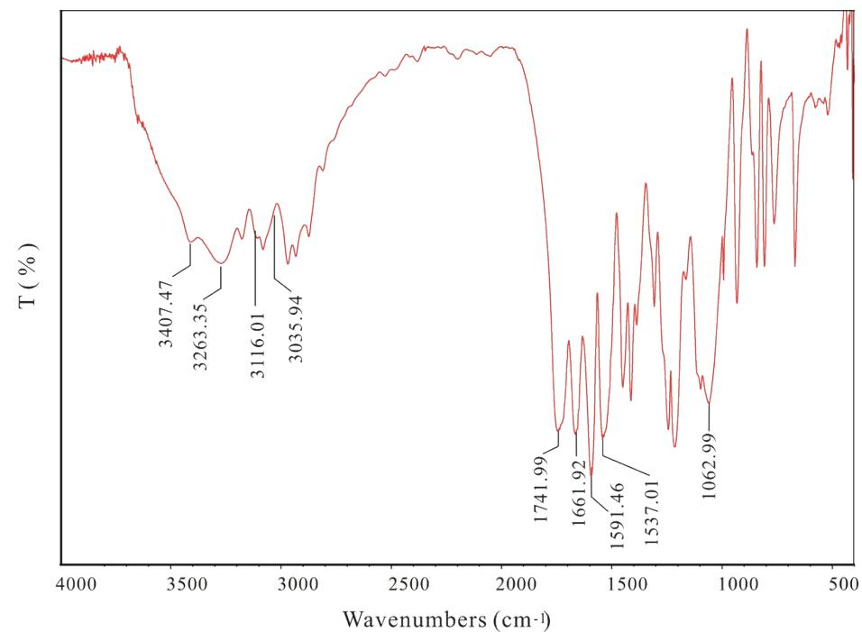
**Fig. S8** IR spectrum of chitosan bis(3,5-dichlorophenylcarbamate)-(isobutyrylamide) (P2)
