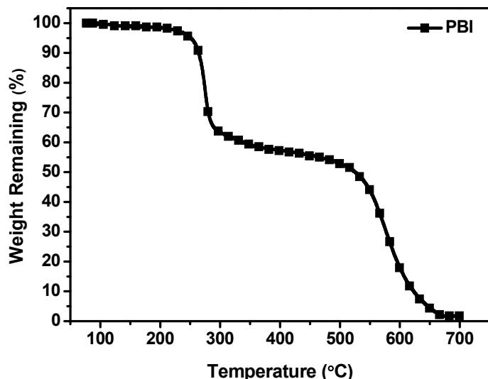
**Fig. S1** TGA curve of **PBI**.
