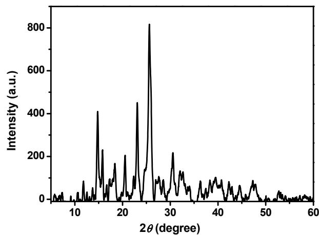
**Fig.S7** XRD patterns of **PBI** nanorods.
