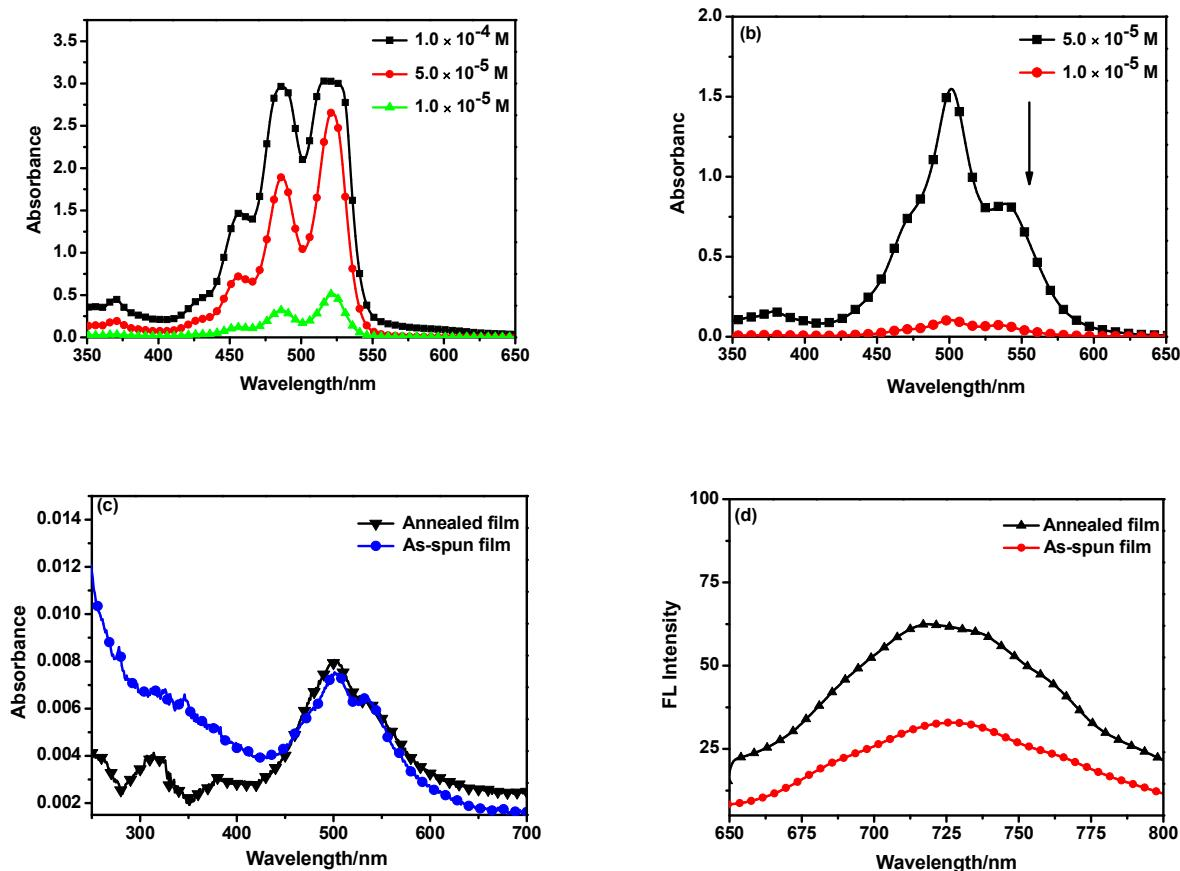
**Fig. S2** Changes in UV-vis absorption spectra of **PBI** (a) in methanol and (b) in water at different concentrations; (c) UV-vis spectra of **PBI** in annealed film and as-spun film; (d) Emission spectra of **PBI** in annealed film and as-spun film.
