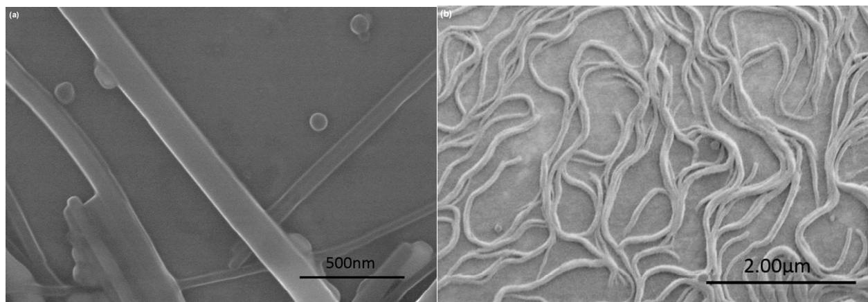
**Fig. S5** (a) SEM image of the nanorods assembled from **PBI** for 4 days in methanol ( $1 \times 10^{-4}$  M); (b) SEM image of nanofibers assembled from **PBI** for 4 days in water ( $1 \times 10^{-4}$  M).
