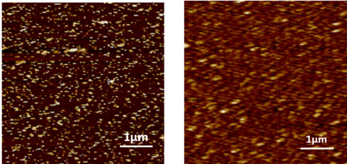
**Fig. S8** AFM topographic images of the solution processed **PBI** films (a) before and (b) after annealed at  $80^\circ\text{C}$  for 1 h. Scan size ( $5 \times 5 \mu\text{m}^2$ ).
