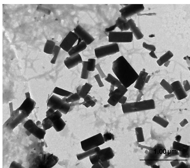
**Fig. S6** TEM image of the nanorods assembled from **PBI** for 4 days in methanol ( $1 \times 10^{-4}$  M).
