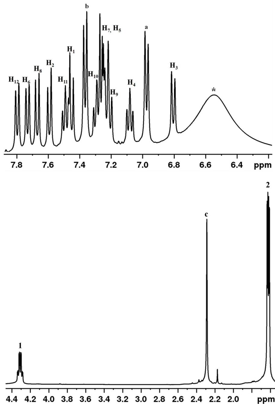
400 MHz TOCSY spectrum of (*R/S*) - 2-Chloro propanoic acid, (*R*)-NOBIN and p-TsOH (1:1:1)
