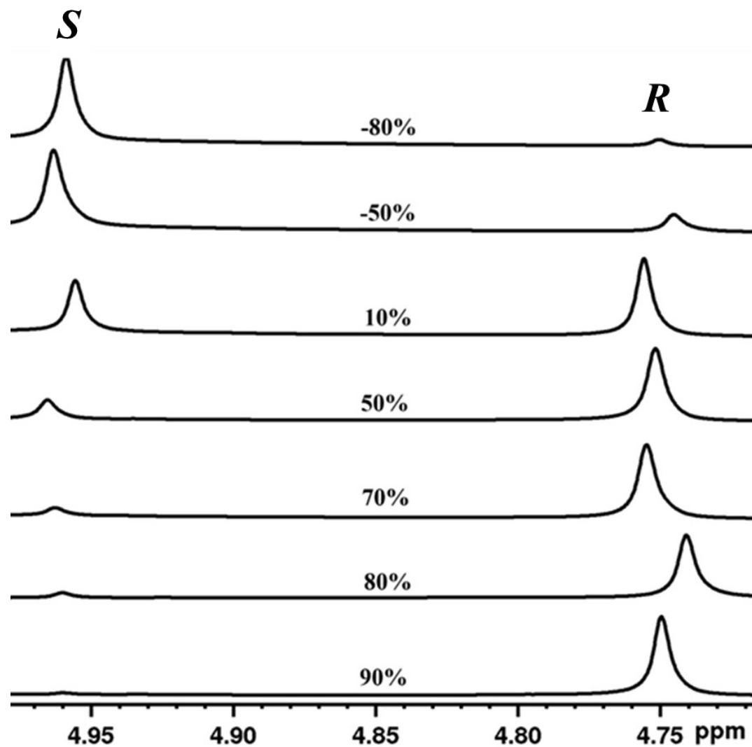
400 MHz  $^1\text{H}$ -NMR spectrum of (*R/S*)-Mandelic acid, (*R*)-NOBIN and Methyl p-Toluenesulfonate in  $\text{CDCl}_3$
