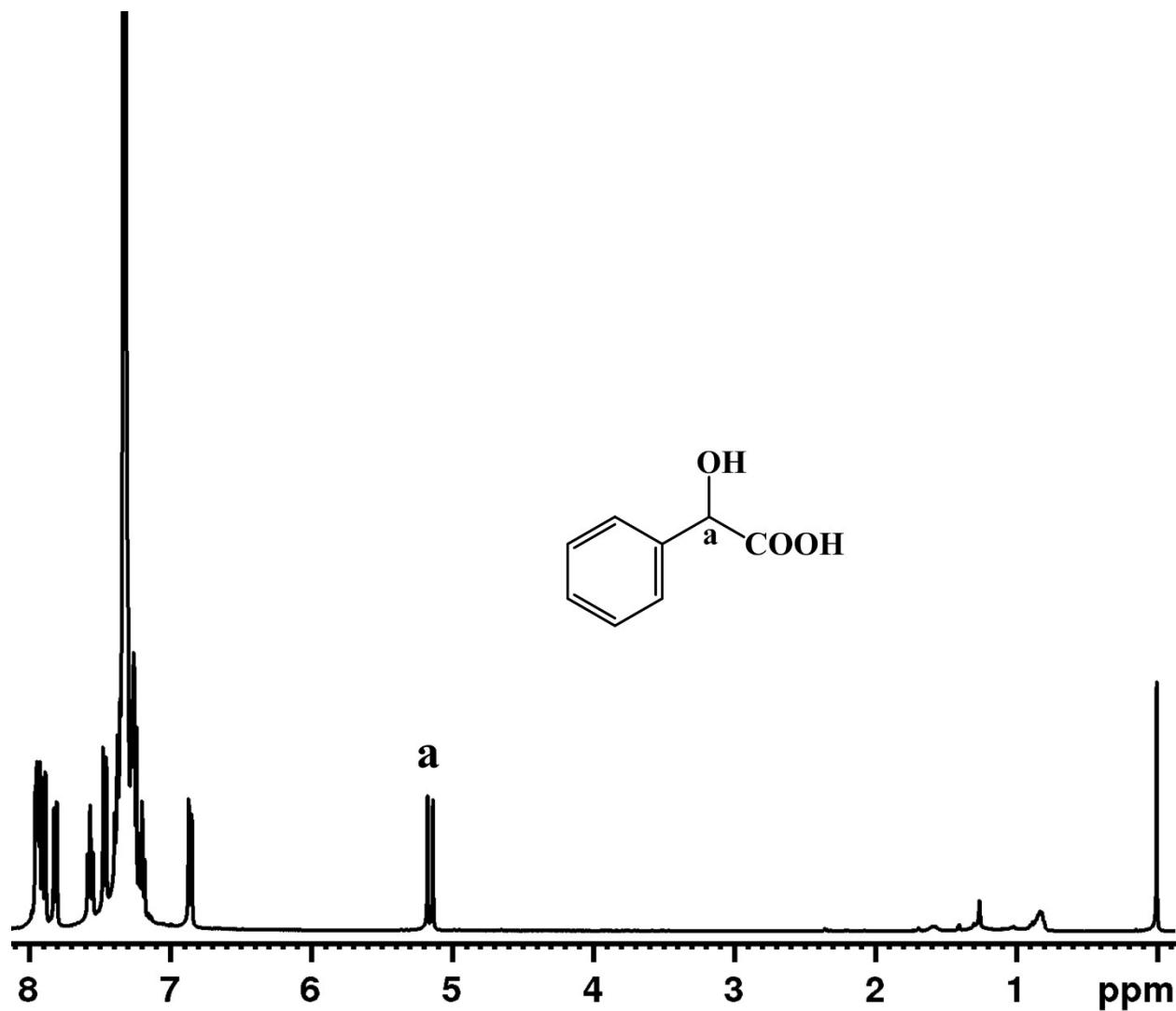
400 MHz  $^1\text{H}$ -NMR spectrum of (*R/S*)-Mandelic acid, (*R*)-NOBIN and p-TsOH in  $\text{CDCl}_3$
