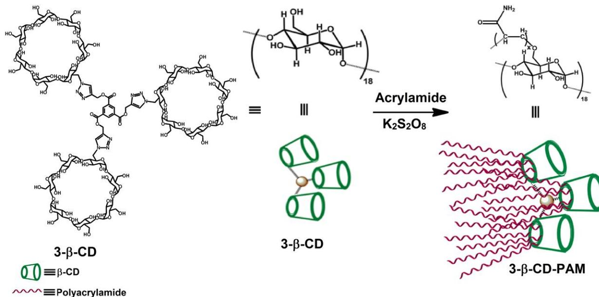
**Scheme S1.** Schematic representation of synthesis of 3-β-CD-PAM.
