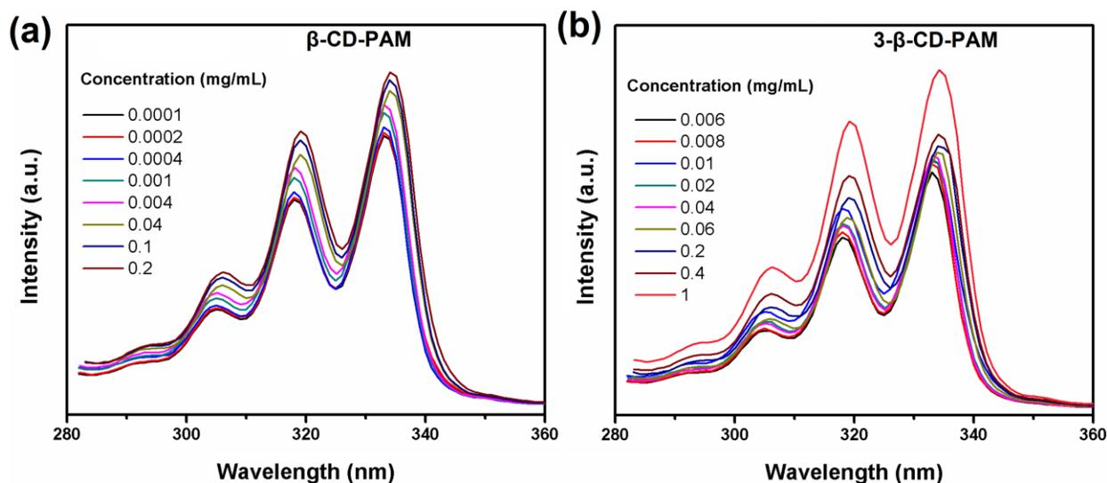
**Fig. S2.** Fluorescence excitation spectra ( $\lambda_{em} = 390$  nm) of pyrene ( $6 \times 10^{-7}$  M) in the presence of progressively higher concentration (C) (mg/mL) of (a)  $\beta$ -CD-PAM and (b) 3- $\beta$ -CD-PAM.
