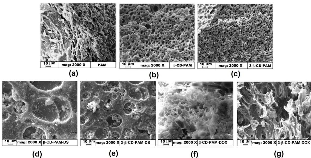
**Fig. S4.** The images from a to g represent the scanning electron micrographs of PAM,  $\beta$ -CD-PAM, 3- $\beta$ -CD-PAM,  $\beta$ -CD-PAM-DS, 3- $\beta$ -CD-PAM-DS,  $\beta$ -CD-PAM-DOX and 3- $\beta$ -CD-PAMDOX respectively.
