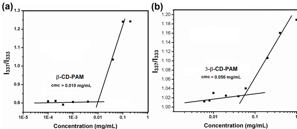
**Fig. S3.** Semi logarithmic plot of the fluorescence excitation intensity ratio ( $I_{337}/I_{333}$ ) of pyrene ( $6 \times 10^{-7}$  M) (monitored at  $\lambda_{em} = 390$  nm) vs the concentration of (a)  $\beta$ -CD-PAM and (b) 3- $\beta$ -CD-PAM, in water.
