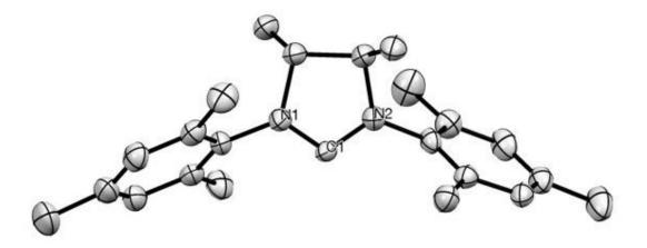
X-Ray diffraction of SIMes<sup>Me-trans</sup>•HCI (CCDC 1487556) indicating the *trans* configuration.
