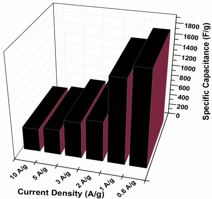
**Fig. S17** Specific Capacitance vs current Density plot of SnS<sub>2</sub>@Cu<sub>2</sub>O/rGO composite
