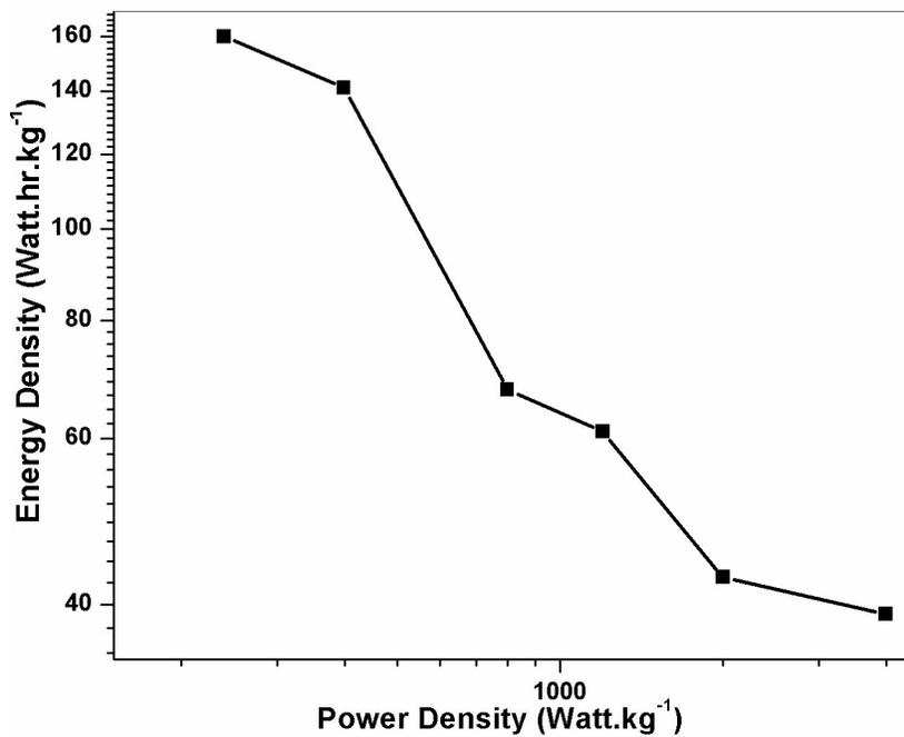
**Fig. S18** Ragone plot of the composite SnS<sub>2</sub>@Cu<sub>2</sub>O/rGO
