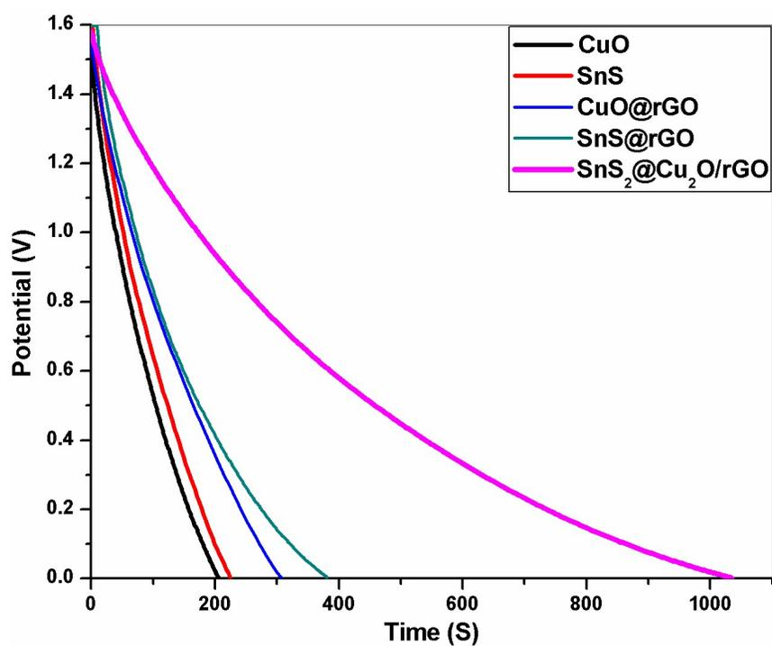
**Fig. S16**GCD curve for various composite along with SnS and CuO in two electrode configuration at the current density 1A/g
