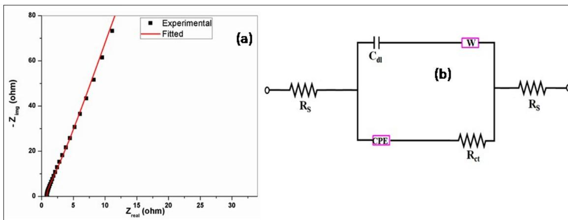
**Fig. S 21 (a)** Nyquist plots of SnS<sub>2</sub>@Cu<sub>2</sub>O/rGO nanocomposite after fitting with an equivalent electrical circuit. **Fig. S 21(b)**Equivalent circuit used for fitting the Nyquist plots
