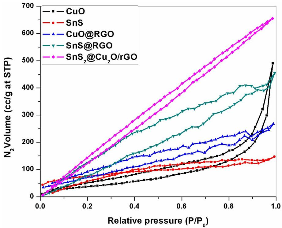
Fig. S15 BET  $N_2$  sorption isotherm for the composites at 77 K
