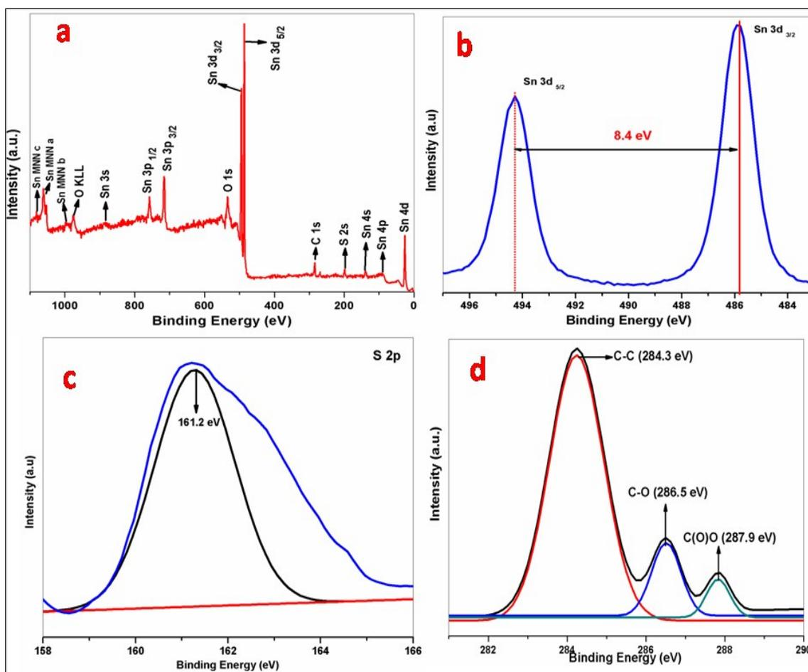
**Fig. S10**XPS (a) Survey spectra of SnS@rGO (b) core level spectra of Sn 3d of SnS@rGO (c) deconvoluted analysis of the S 2p core level spectra of SnS@rGO (d) C 1s core level spectra of SnS@rGO.
