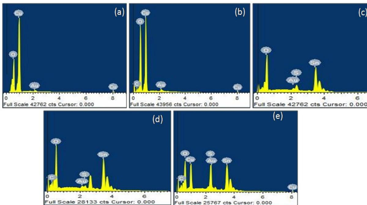
**Fig. S2 (a-e)** Represents the EDS images of (a) CuO nanoparticle (b) CuO@rGO composite (c) SnS (d) SnS@rGO composite (e) SnS<sub>2</sub>@Cu<sub>2</sub>O/rGO composite
