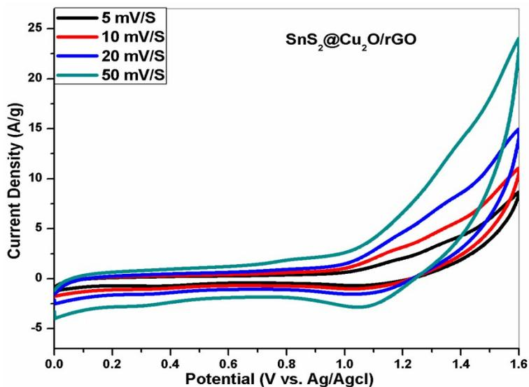
Fig. S13 CV plot of SnS<sub>2</sub>@Cu<sub>2</sub>O/rGO at different scan rate in two electrode organic electrolyte configuration
