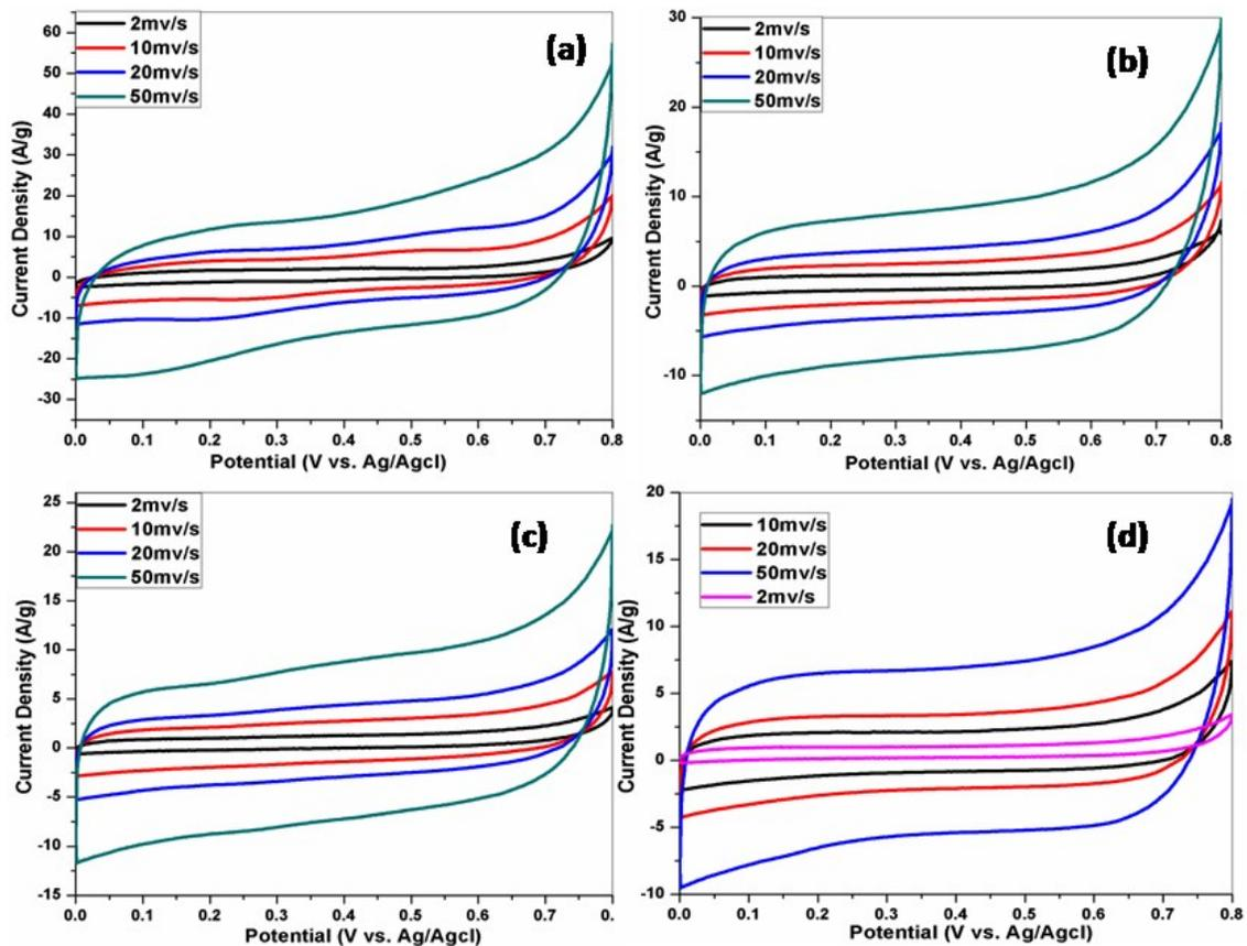
Fig. S12 CV curve at different scan rate for (a) SnS@rGO (b) CuO@rGO (c) SnS (d) CuO
