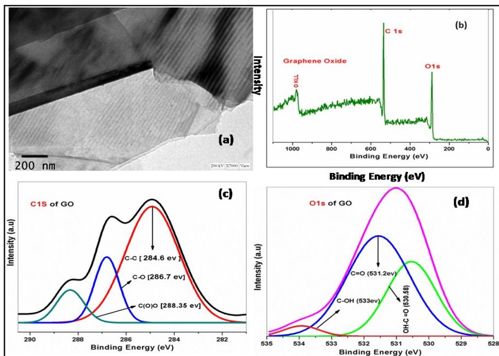
**Fig. S7**(a) TEM of GO (b) XPS survey spectra of GO (c) C 1s of GO (d) O 1s of GO
