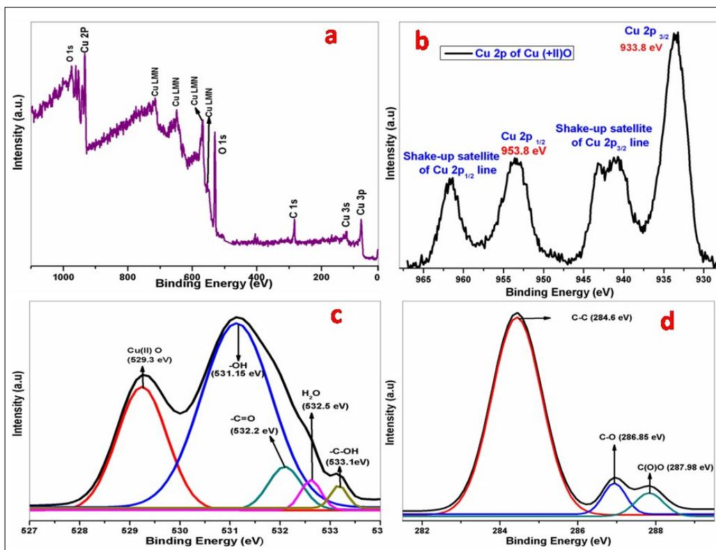
**Fig. S8**XPS (a) Survey spectra of CuO@rGO (b) core level spectra of Cu 2p of CuO@rGO (c) deconvoluted analysis of the O1s core level spectra of CuO@rGO (d) C1s spectra of CuO@rGO.
