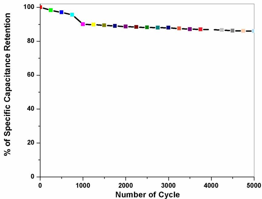
Fig. S20 Retention of specific capacitance for the composite SnS<sub>2</sub>@Cu<sub>2</sub>O/rGO composite at current density 1 A/g in three electrode system upto 5000 cycles
