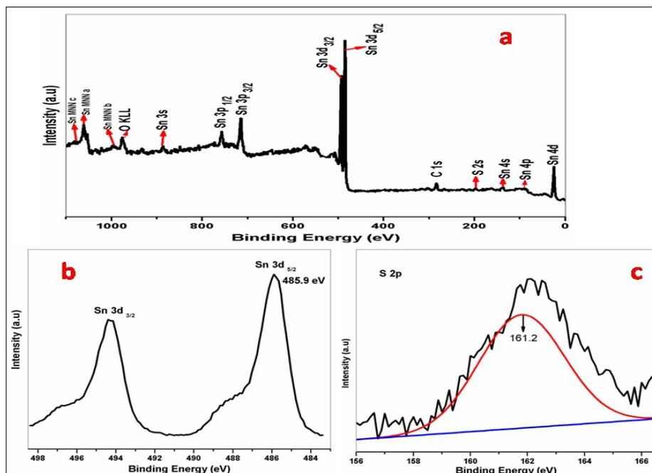
**Fig. S9**XPS (a) Survey spectra of SnS (b) core level spectra of Sn 3d of SnS (c) deconvoluted analysis of the S2p core level spectra of SnS.
