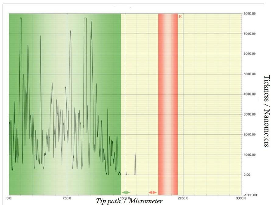
**Figure S12.** Profilometric view of a screen-printed NiO photocathode.
