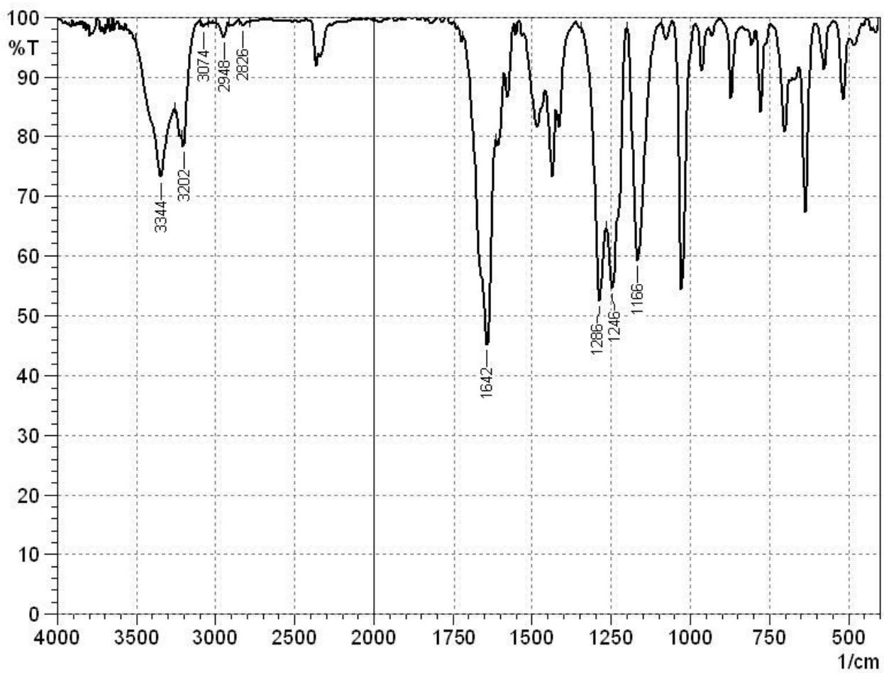
**Figure 44S.** IR spectrum of  $[4\mathbf{a}(\text{OTf})_2]$ .
