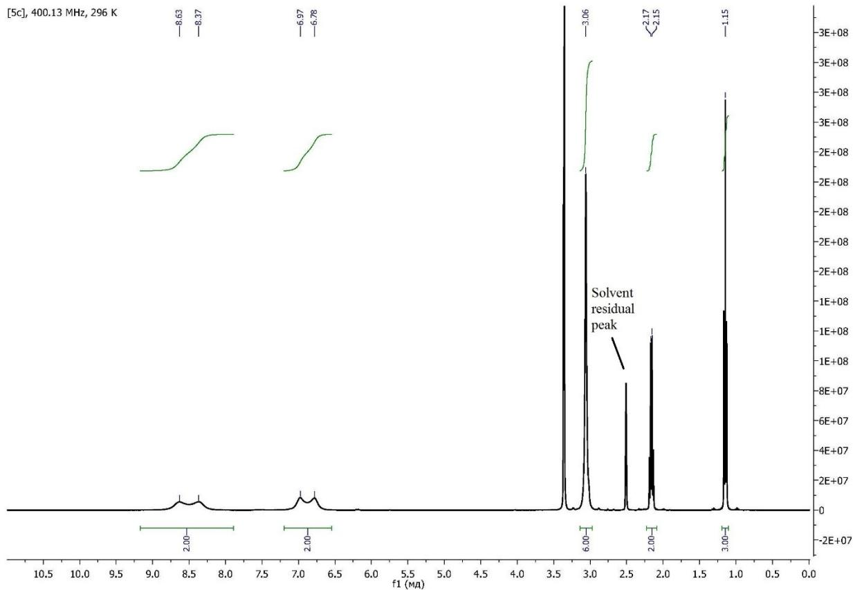
**Figure 70S.**  $^1\text{H}$  NMR spectrum of [5c](OTf).
