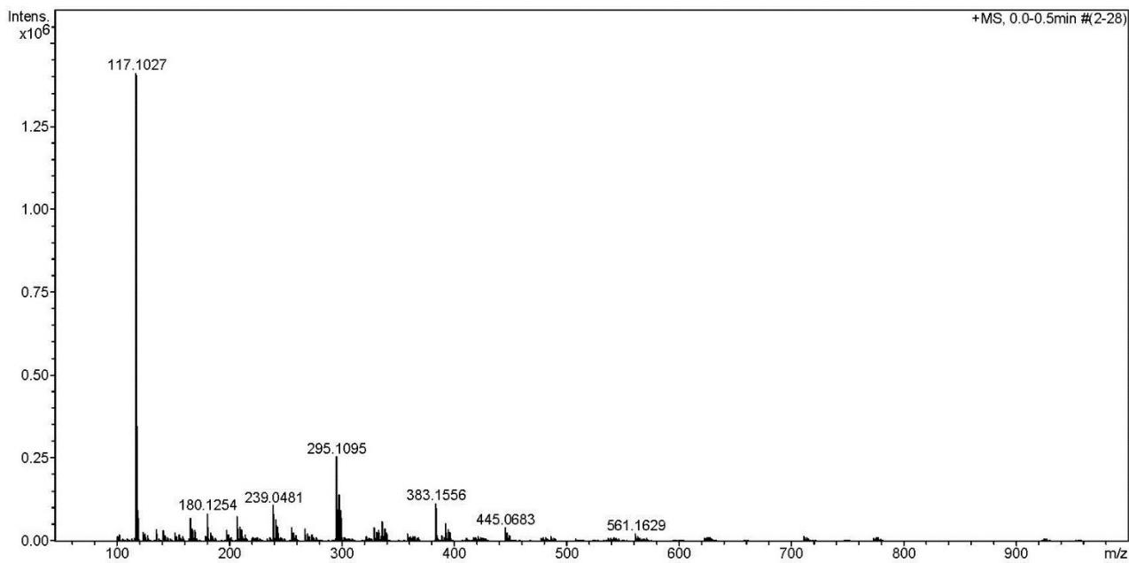
Figure 37S. Positive mass-spectrum of [3d](OTf)<sub>4</sub>.
