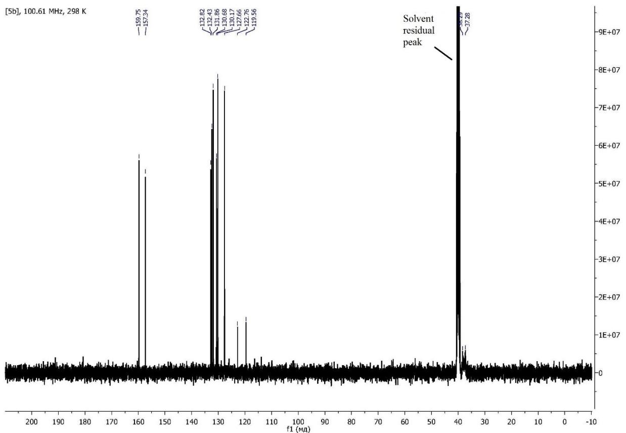
**Figure 66S.**  $^{13}\text{C}$  NMR spectrum of [5b](OTf).
