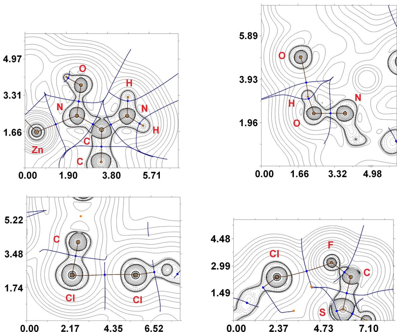
**Figure 77S.** Contour line diagrams of the Laplacian distribution  $\nabla^2\rho(\mathbf{r})$ , bond paths and selected zero-flux surfaces for HB's in **2a** (top) and XB's in **2b** (down left) and **[4b(OTf)(EtOH)](OTf)** (down right). Bond critical points (3, -1) are shown in blue, nuclear critical points (3, -3) – in pale brown, ring critical points (3, +1) – in orange, length unit – Å.
