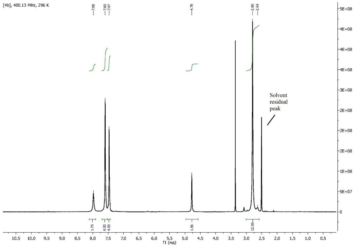
**Figure 50S.**  $^1\text{H}$  NMR spectrum of  $[\mathbf{4b}(\text{OTf})_2]$ .
