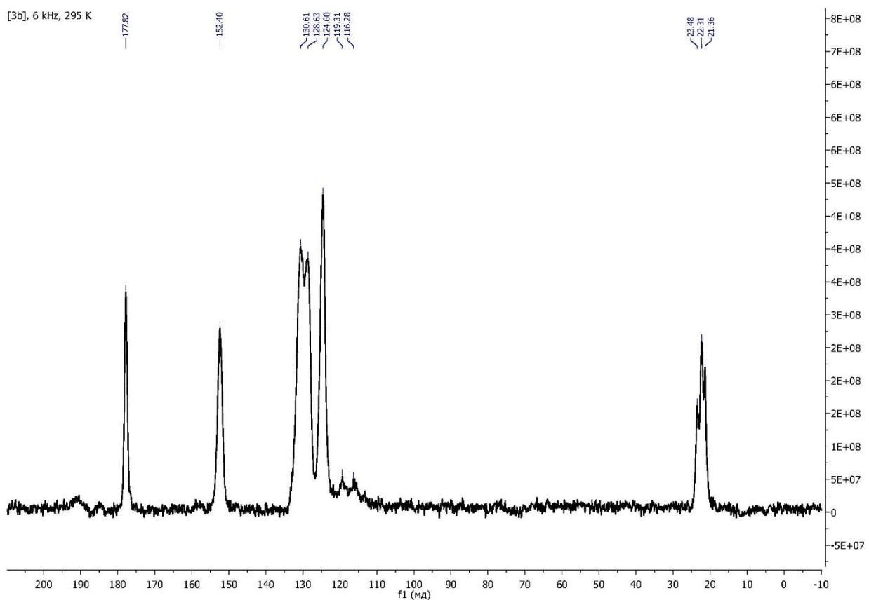
**Figure 31S.**  $^{13}\text{C}\{^1\text{H}\}$  CP-MAS TOSS NMR spectrum of  $[\mathbf{3b}](\text{OTf})_4$ .
