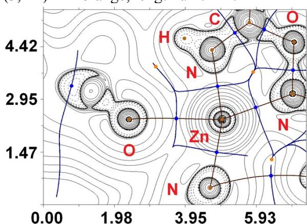
**Figure 77S.** Contour line diagram of the Laplacian distribution  $\nabla^2\rho(\mathbf{r})$ , bond paths and selected zero-flux surfaces for contacts Zn–O and Zn–N in **[4c(OTf)<sub>2</sub>]**. Bond critical points (3, -1) are shown in blue, nuclear critical points (3, -3) – in pale brown, ring critical points (3, +1) – in orange, length unit – Å.
