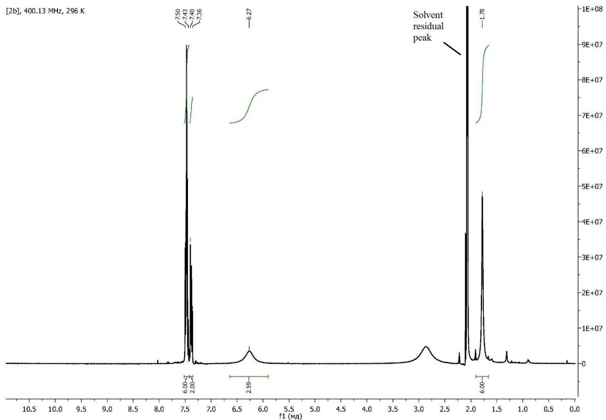
**Figure 10S.**  $^1\text{H}$  NMR spectrum of **2b**.
