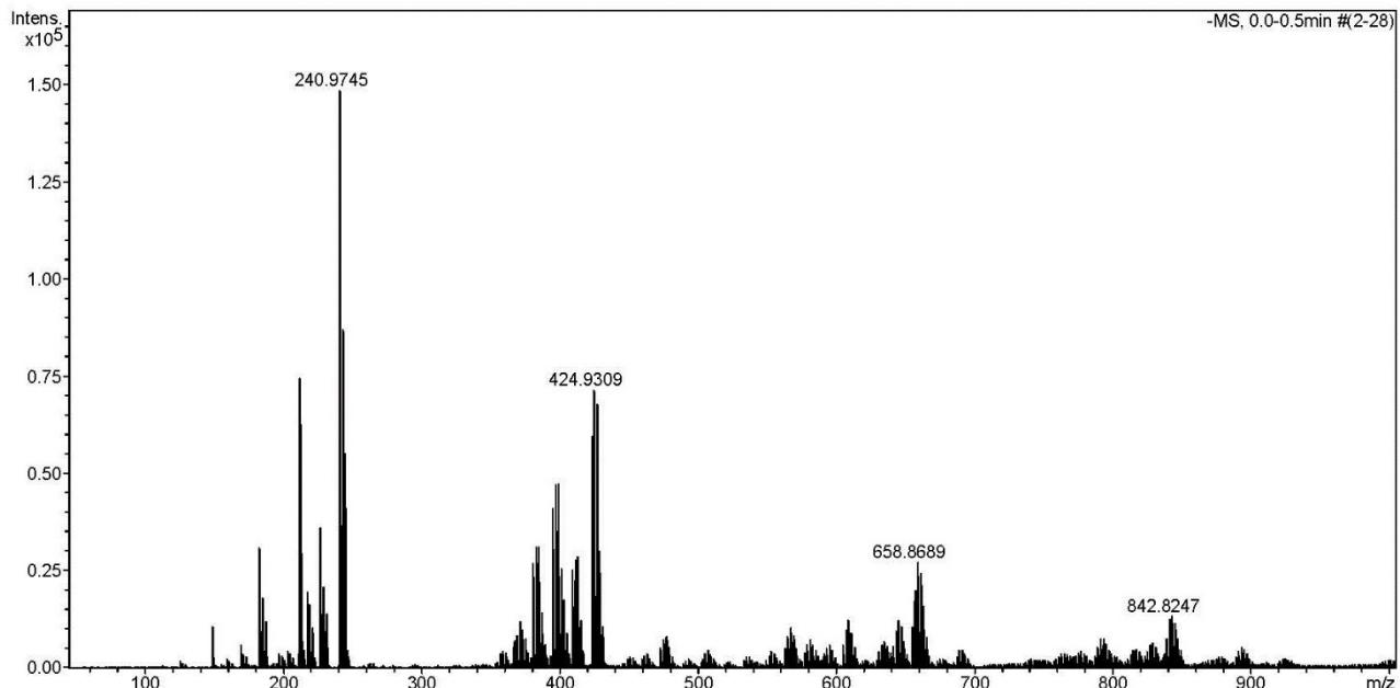
Figure 8S. Negative mass-spectrum of 2b.
