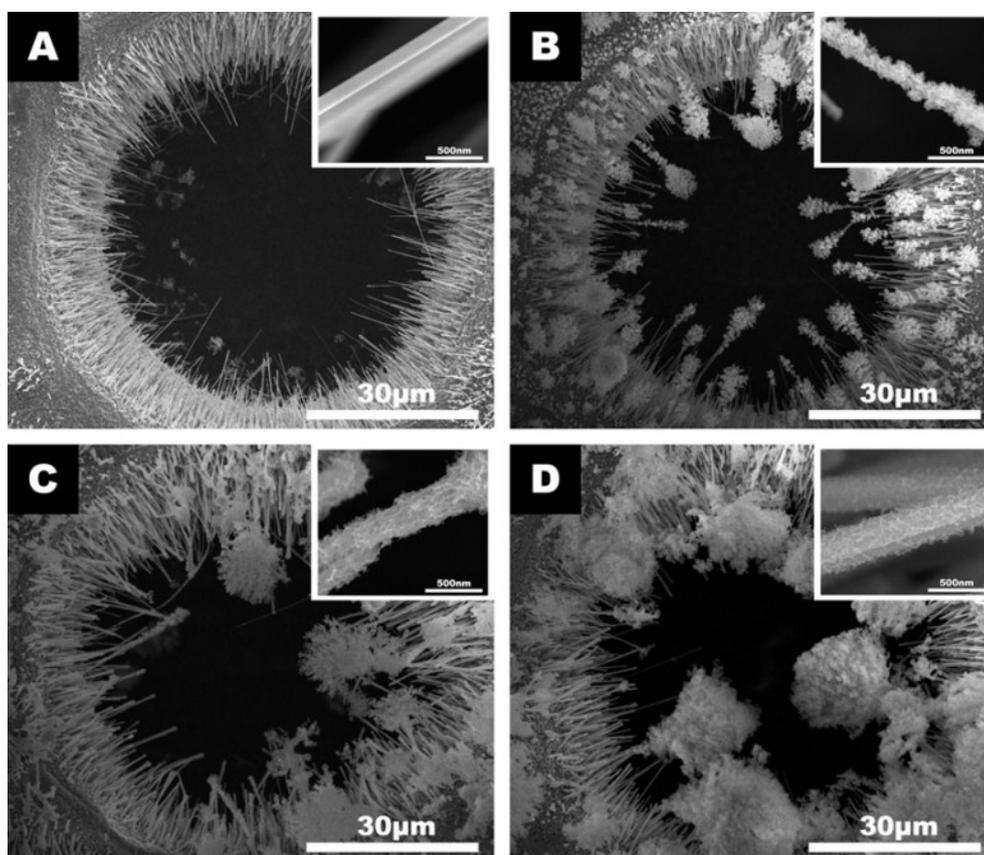
**Fig. S-2** The SEM images of the CuO/Ag Nano-dandelion prepared with different deposition time. The precursor concentration is 10 mM. The typical deposition current was 150 nA A) 5 min; B) 15min; C) 30 min; D) 60 min.
