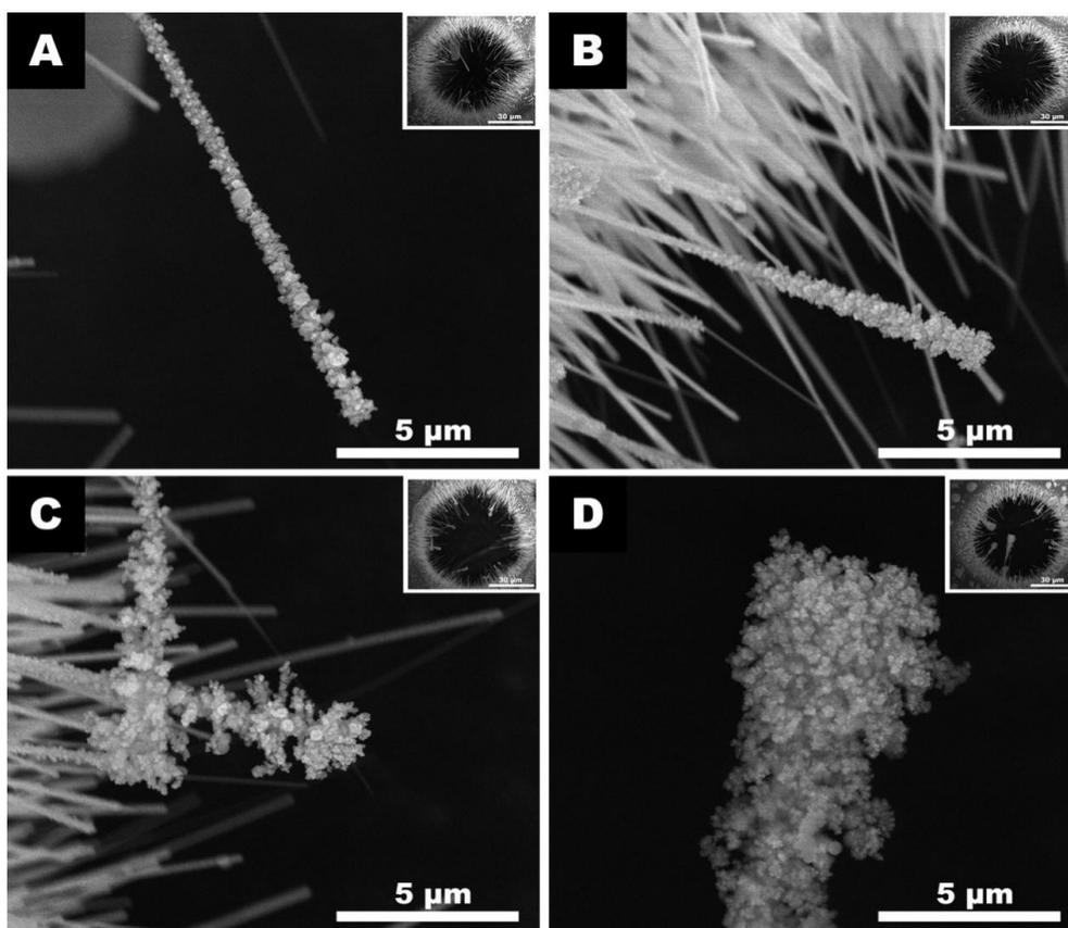
**Fig. S-3** The SEM images of the CuO/Ag Nano-dandelion prepared with different deposition currents. The precursor concentration is 10 mM and the deposition time is 15 min. A) 10 nA; B) 50 nA; C) 100 nA; D) 150 nA.
