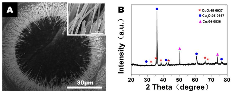
**Fig. S-1** The CuO nanowires prepared with the thermal oxidation method. A) the SEM image and B) the XRD pattern.
