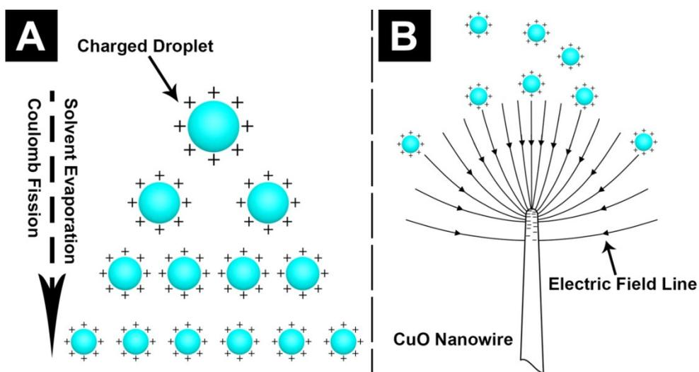
**Fig. S-4** A) The schematic representation of Coulomb fission process of charged microdroplets, B) schematic representation of microdroplets soft-landed onto the CuO nanowires driven by the electric field force.
