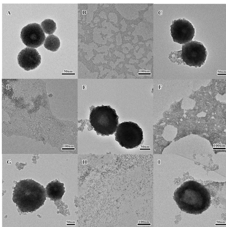
**Fig. S3** TEM images of reversible changes on morphology induced by NaOH and HCl. (A) 1<sup>st</sup>, assembly; (B) 1<sup>st</sup>, disassembly; (C) 2<sup>nd</sup>, assembly; (D) 2<sup>nd</sup>, disassembly; (E) 3<sup>rd</sup>, assembly; (F) 3<sup>rd</sup>, disassembly; (G) 4<sup>th</sup>, assembly; (H) 4<sup>th</sup>, disassembly; (I) 5<sup>th</sup>, assembly.
