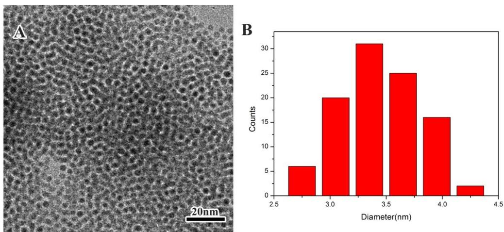
**Fig. S1** TEM image (A) and size distribution (B) of Au NPs capped with OL ( $3.4 \pm 0.3$  nm).
