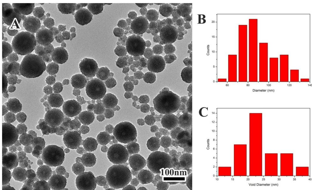
**Fig. S2** (A) TEM image of self-assembled Au NVs and size distributions of (B) vesicles ( $89.2 \pm 16.8$  nm) and (C) voids in NVs ( $23.4 \pm 6.5$  nm).
