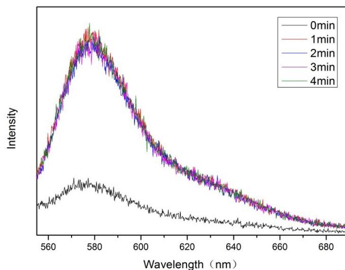
**Fig. S4** Fluorescence emission spectra of RhB released from Au NVs after addition of a certain amount of NaOH over time.
