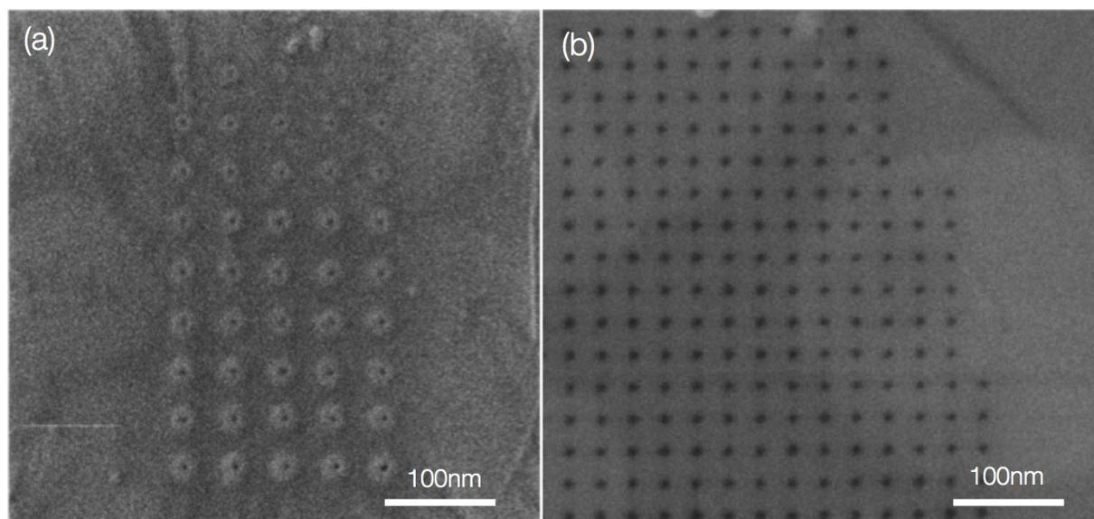
**Figure S2.** He<sup>+</sup> ion micrograph of etched pores in HIM. **(a)** Probe current of 1.4 pA and dwell times from 100 ms to 4600 ms (top to bottom row in steps of 500 ms). Strong deposition of material is visible around each patterned feature. Only beam-irradiation dwell times higher than 1600 ms show pores clearly visible in the micrograph. **(b)** Probe current of 10.5 pA with a dwell time of 15 ms leads to pore formation with no deposition in the vicinity of it.
