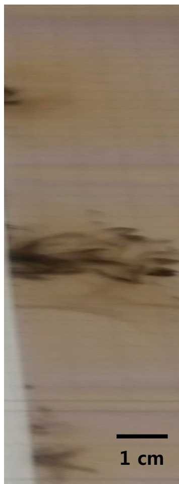
Fig. S5 Image of the film that was partially damaged due to excessive energy absorption from a large-area IPL overlap.
