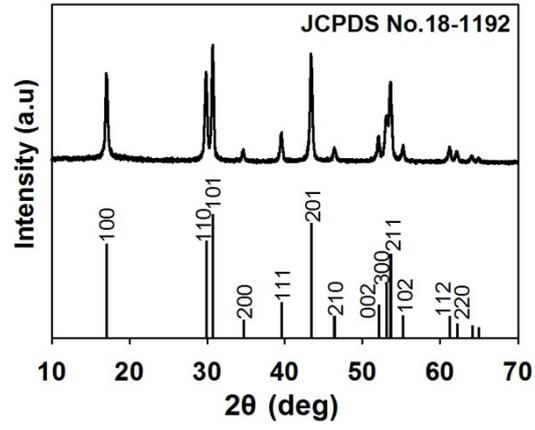
**Fig. S3.** XRD spectrum of OA-capped NaYF<sub>4</sub>:Yb,Tm@NaYF<sub>4</sub> core-shell nanocrystals.
