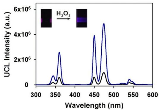
**Fig. S10.** UCL spectrum of DNA-AgNPs/UCNP before (black) and after (blue) incubation with 500  $\mu\text{M}$   $\text{H}_2\text{O}_2$  for 80 min. The photos displaying change in the blue UCL emissions under the 980 nm excitation.
