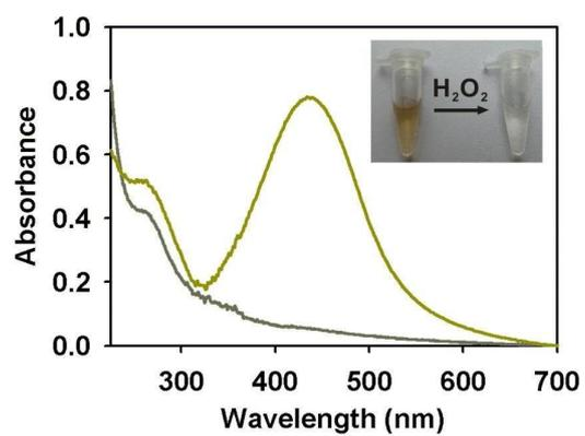
**Fig. S9.** Absorption spectra of DNA-templated AgNPs before (yellow) and after (grey) addition of 500  $\mu$ M  $H_2O_2$ .
