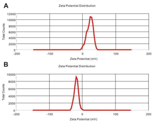
**Fig. S5.**  $\zeta$ - potential analysis of (A) the bare UCNPs and (B) DNA-AgNPs/UCNP. After the attachment of DNA-AgNPs, the  $\zeta$ -potentials of the bare UCNPs changed from +22.5 mV to -18 mV (pH 7.0), as a result of increased number of DNA-AgNPs on the UCNPs surface.
