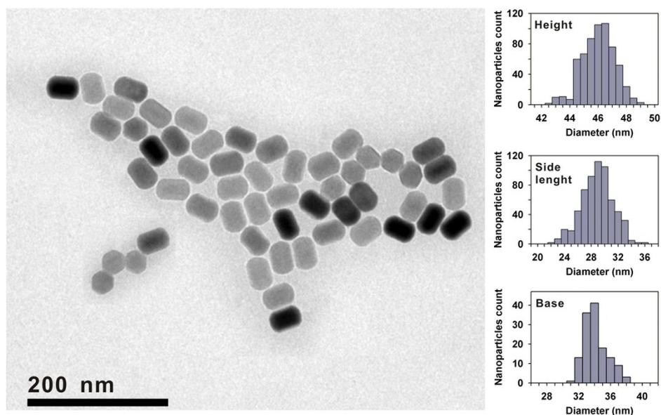
**Fig. S2.** TEM images and histograms of OA-capped NaYF<sub>4</sub>:Yb/Tm@NaYF<sub>4</sub> core-shell nanocrystals.
