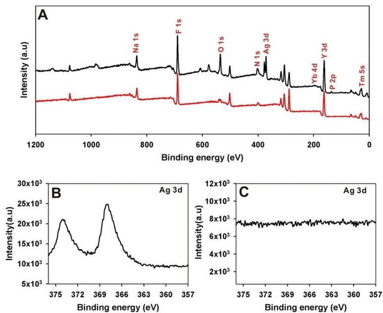
**Fig. S8.** (A) XPS spectrum of OA-UCNPs (red) and DNA-AgNPs/UCNP nanocomposite (black). (B) High resolution Ag (3d) XPS spectrum of DNA-AgNPs/UCNP nanocomposite. (C) High resolution Ag (3d) XPS spectrum of OA-UCNPs.
