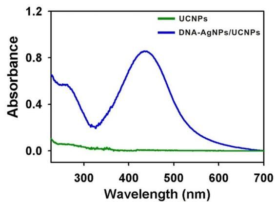
**Fig. S6.** UV-vis absorption spectra of the bared UCNPs (green) and DNA-AgNPs/UCNP nanocomposite (blue).
