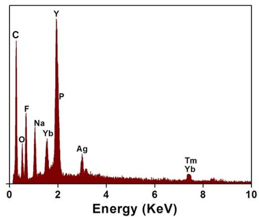
**Fig. S7.** EDS spectrum of DNA-AgNPs/UCNP nanocomposite.
