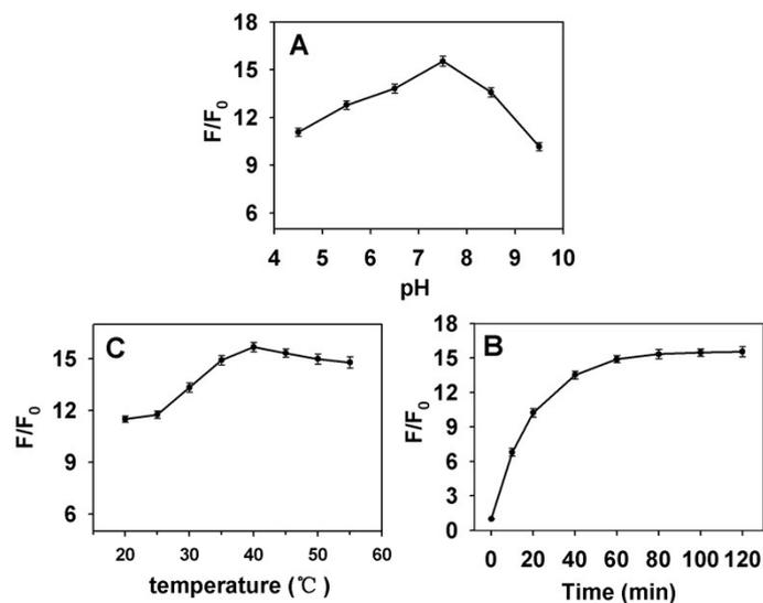
**Fig. S11.** Effects of pH value (A), temperature (B) and incubation time (C) on the upconversion fluorescence enhancement of DNA-AgNPs/UCNP in the absence and presence of 500  $\mu\text{M}$   $\text{H}_2\text{O}_2$ .  $F_0$  and  $F$  represent the UCL intensity of nanocomposite before and after mixing with  $\text{H}_2\text{O}_2$ , respectively. Error bars signify standard deviation (SD) of three independent measurement.
