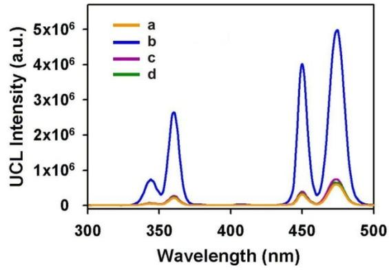
**Fig. S12.** UCL spectrum of (a) DNA-AgNPs/UCNP in the presence of (b) glucose + GOx; (c) GOx; (d) glucose. Conditions: glucose, 400  $\mu$ M; GOx, 25  $\mu$ g/mL; DNA-AgNPs/UCNP, 0.05 mg/mL.
