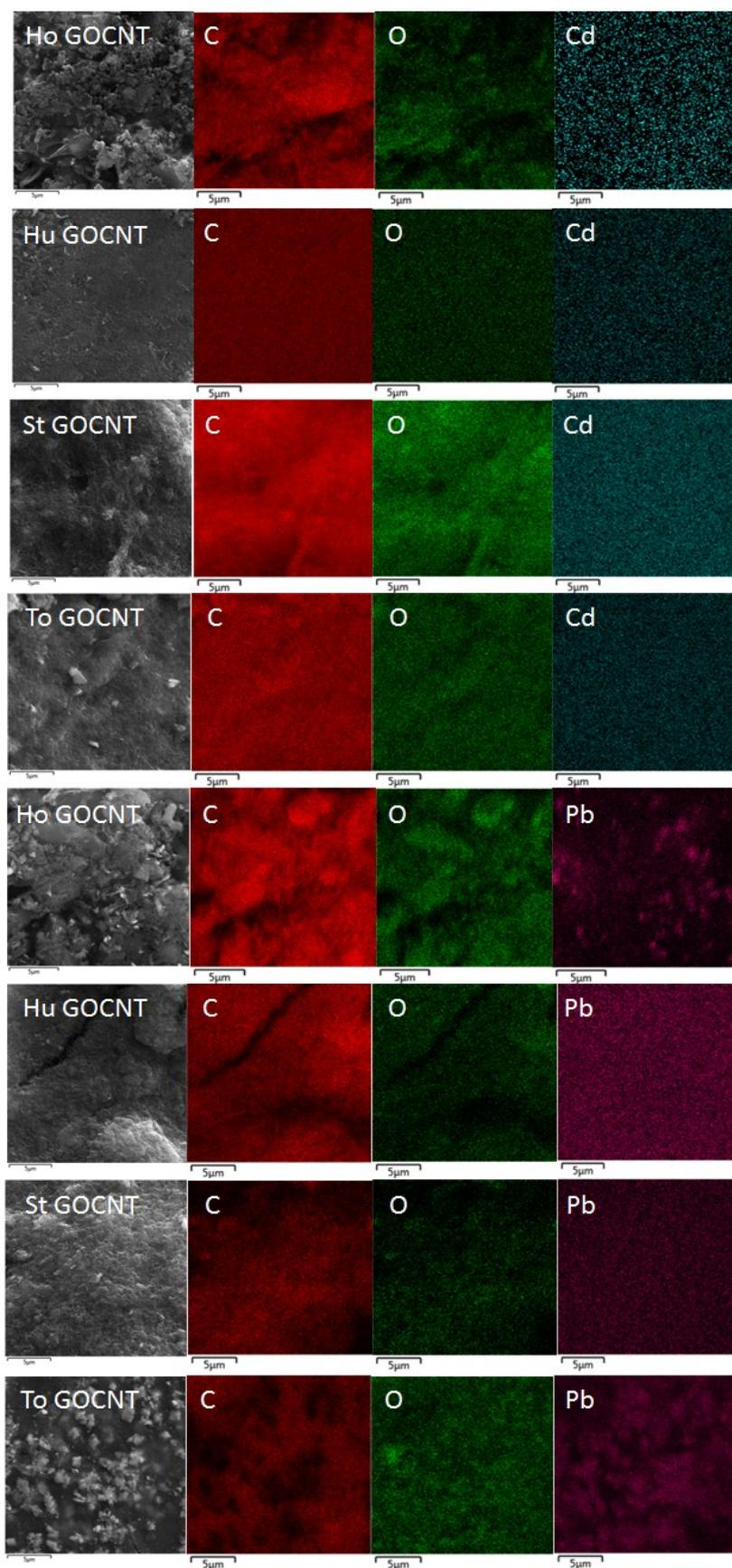
**Fig. S7.** Elemental maps of nanocables after sorption of cadmium and lead.
