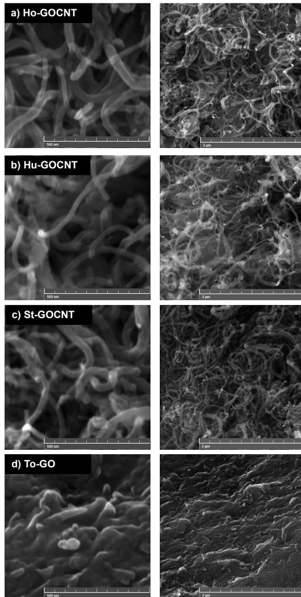
**Fig. S2** Scanning electron micrographs of GOCNT resulting from oxidative opening of CNT prepared by Hofmann (Ho-GOCNT), Hummers (Hu-GOCNT), Staudenmaier (St-GOCNT) and Tour (To-GO, d) methods at different magnifications.
