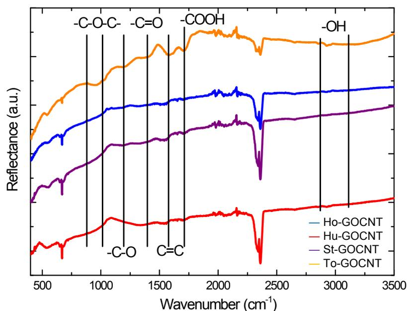
**Fig. S5** FTIR spectra the different hybrid GOCNT nanomaterials.
