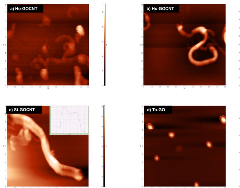
**Fig. S4** AFM images of GOCNT resulting from oxidative opening of CNT prepared by Hofmann (Ho-GOCNT), Hummers (Hu-GOCNT), Staudenmaier (St-GOCNT) and Tour (To-GO, d) methods at different magnifications.
