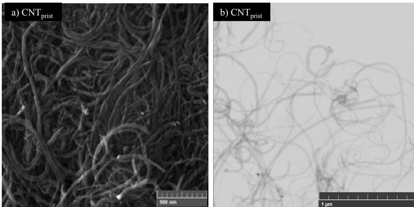
**Fig. S1** SEM (a) and STEM (b) of starting material CNT<sub>prist</sub>.
