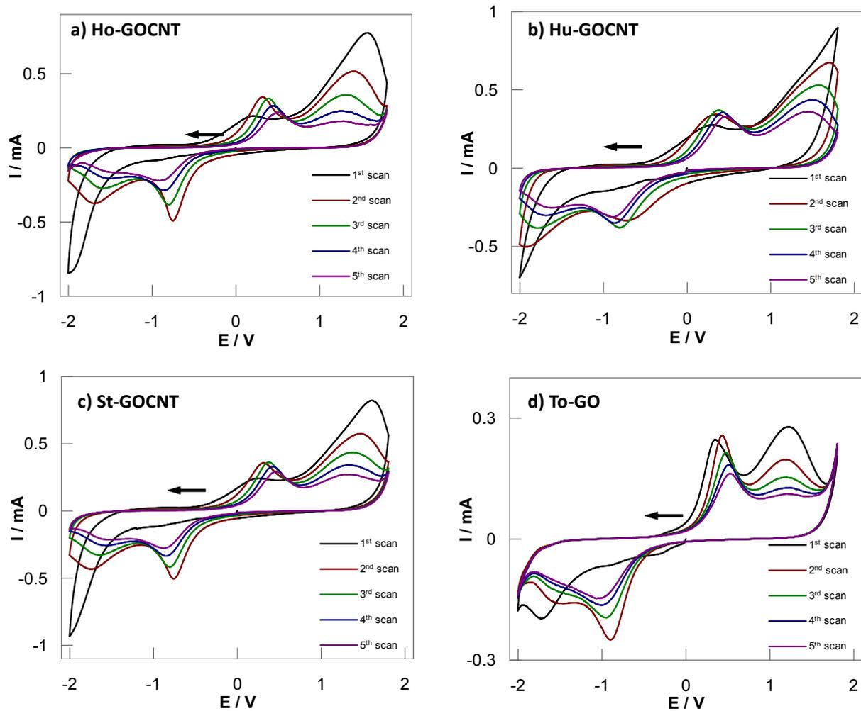
**Fig. S6.** CVs of GOCNT prepared through the methods of a) Hummers, b) Hofmann, c) Staudenmaier, d) Tour. Arrows indicate the directions of the first scans (towards reducing potentials). All starting potentials are 0.0 V and are relative to the Ag/AgCl reference electrode. Supporting electrolyte: 0.1 M PBS at pH 7.2; scan rate: 100 mV/s.
