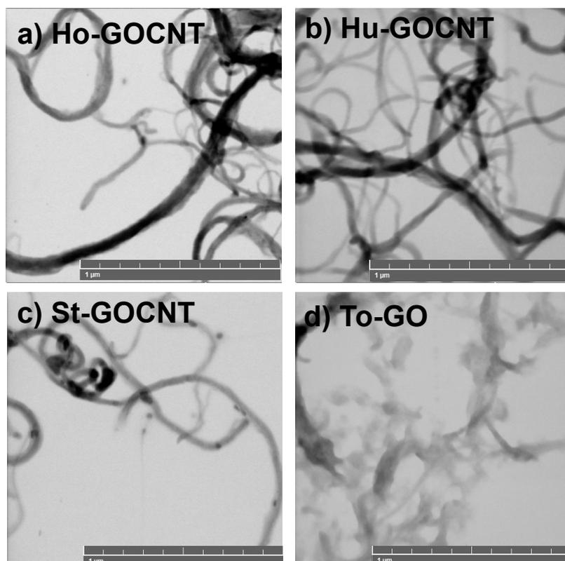
**Fig. S3** Scanning transmission electron micrographs (STEM) of GOCNT resulting from oxidative opening of CNT prepared by Hofmann (Ho-GOCNT), Hummers (Hu-GOCNT), Staudenmaier (St-GOCNT) and Tour (To-GO, d) methods at 100K magnifications.
