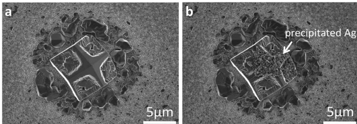
Fig. S3. The whole surface of the sulfurised Ag-layer is covered with Ag<sub>2</sub>S crystals. a): A large Ag<sub>2</sub>S crystal. b): SEM observation caused Ag precipitation on the surface of the large Ag<sub>2</sub>S crystals, when magnification was increased in the meanwhile of image a) and b).
