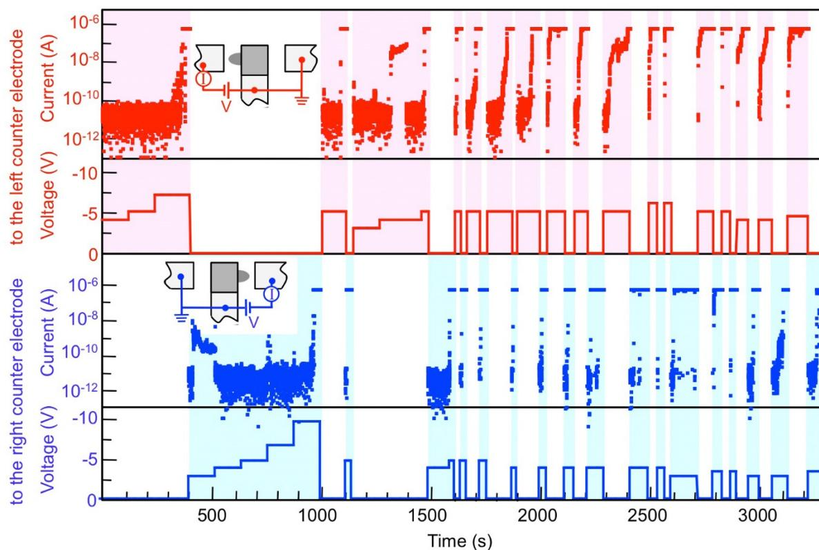
Fig. S5. Same data as in Figure 4 of the main manuscript with log scale for the current. It can be seen that the current always started in the range of pA, showing that the connections were broken before being re-established.
