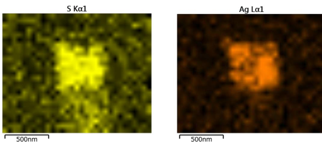
Fig. S1. EDS data: Continuous layer of Ag<sub>2</sub>S for small electrodes; S around electrode due to thiophene containing polymer on sample.
