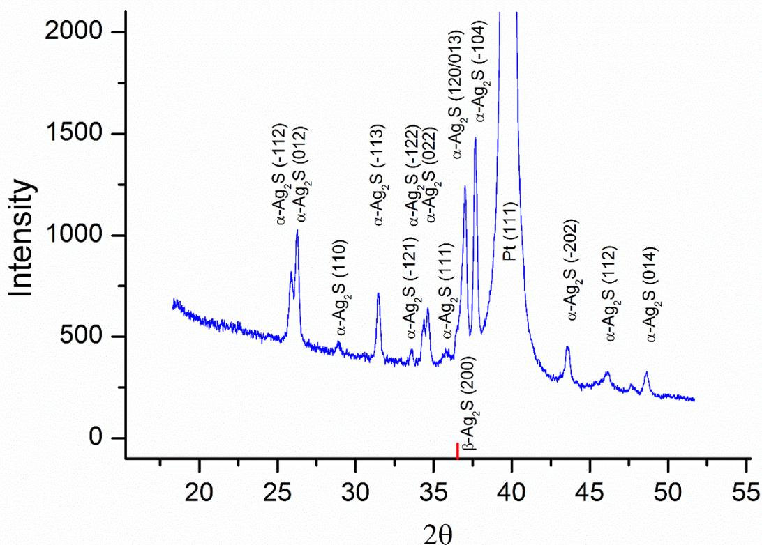
Fig. S4. XRD data for the Ag<sub>2</sub>S film formed by the same process used for the device fabrication. Observed peaks indicate that the Ag<sub>2</sub>S is in  $\alpha$ -phase.
