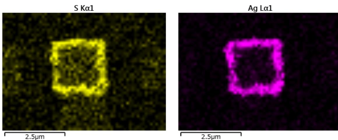
Fig. S2. For larger electrodes, Ag was moved away of original position during sulfurisation, resulting in a continuous border of Ag<sub>2</sub>S around the electrodes. Complete areal overlap of the signals from Ag and S indicates that all Ag was sulfurised.
