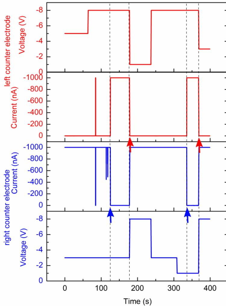
Fig. S6. Disconnection induced by establishment of connection to the opposite side. All of the four disconnections, indicated by arrows, occurred at the exact moment when connection to the other side was established. For example, the disconnections indicated by blue arrows occurred when the connection to the left counter electrode was established. At this time, the bias voltage applied to the right counter electrode was constant and smaller than the bias to the left counter electrode.
