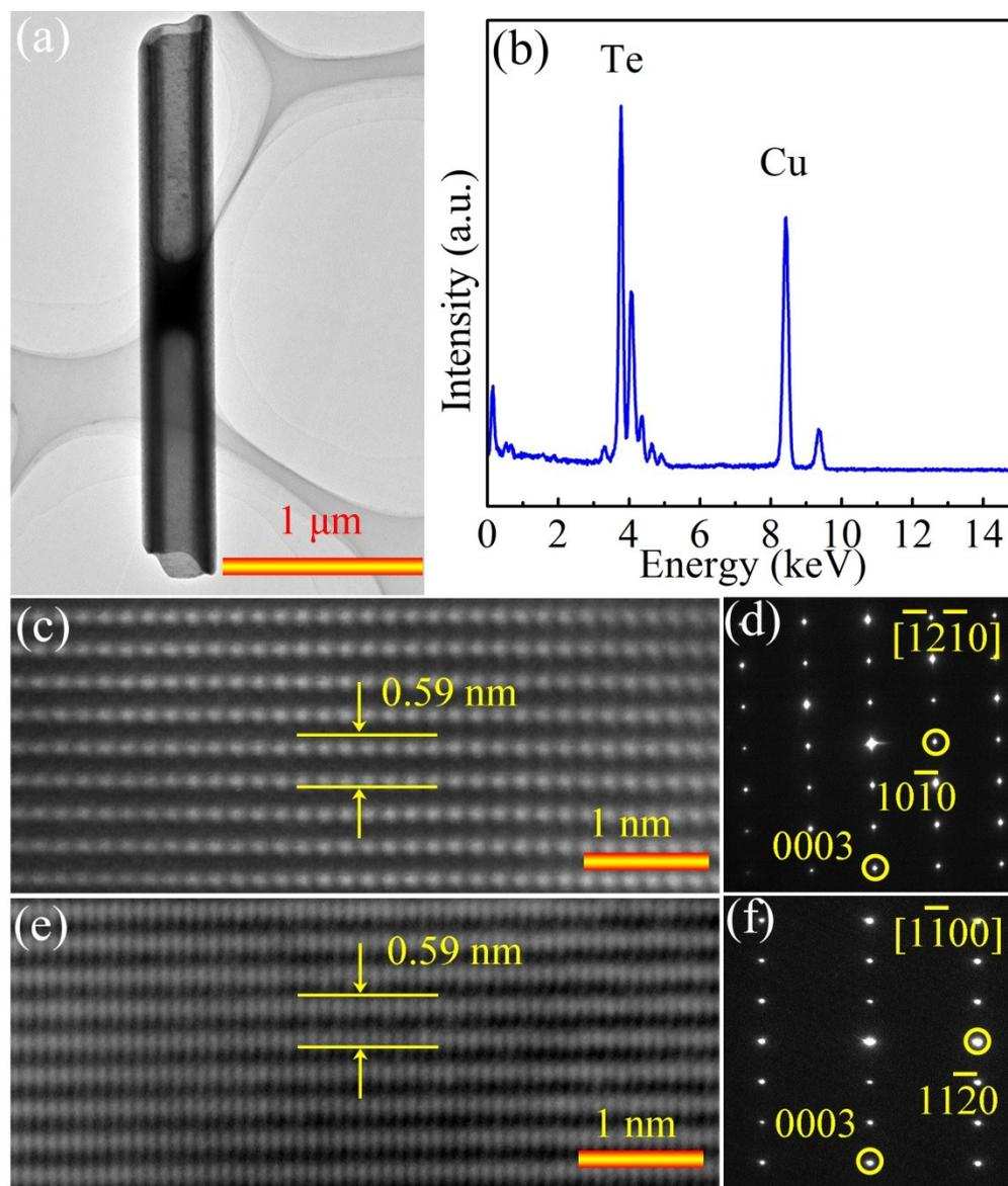
Fig. S3 (a) TEM image of a typical Te nanotube. (b) EDS profile taken from this Te nanotube. (c) HRTEM, and (d) corresponding  $[\bar{1}2\bar{1}0]$  zone-axis SAED pattern. (e) HRTEM, and (f) corresponding  $[1\bar{1}00]$  zone-axis SAED pattern.
