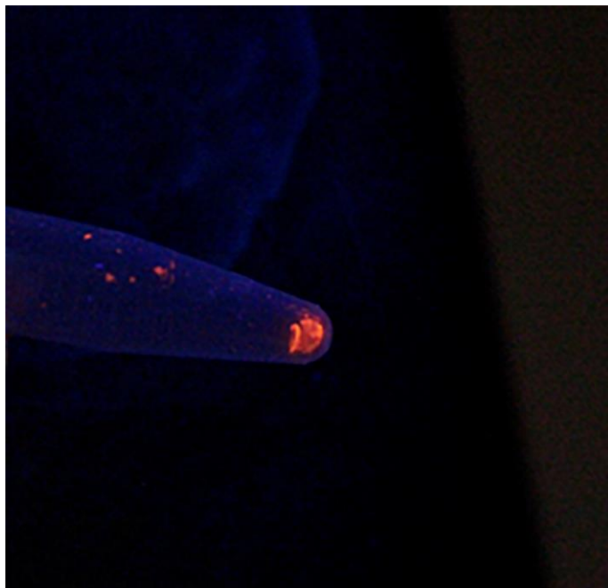
Figure S2. Digital photograph of the nanoparticles pellet excited with a UV lamp (254 nm) shows typical red emission from \text{Eu}^{3+} ions.
