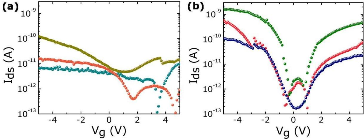
**Figure S1.** Transfer characteristics ( $I_{ds}$ - $V_g$ ) across p-n junction diode at (a)  $V_{ds} = 0.1$  V and (b)  $V_{ds} = 1$  V.
