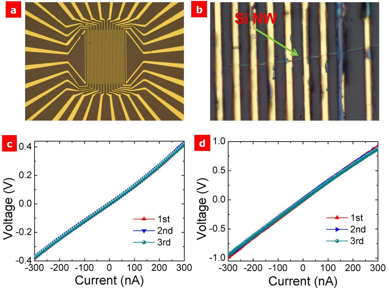
**Figure S2.** Optical images and electrical four-probe transport characteristics of p-n Si NW FETs. (a, b) Optical images of p-n Si NW FET devices. Four-probe voltage–current measurements of the (c) p-type region and (d) n-type region of the p-n Si NW FETs.
