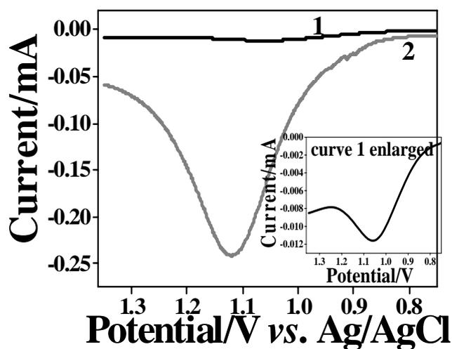
**Figure S-6.** LSV obtained with ITO/PEI/AuNPs of different diameters for 1 h: 1 – 10 nm, and 2 – 40 nm in 0.1 M KCl at a scan rate of  $0.05 \text{ V s}^{-1}$ .
