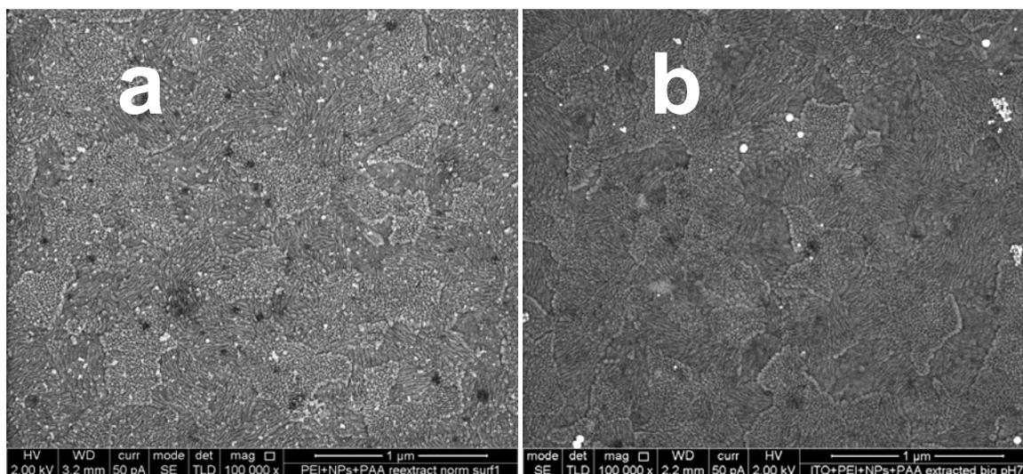
**Figure S-12.** Morphology images of ITO/PEI/SEM images of ITO/PEI/PAA imprinted by 10 nm AuNPs, after reuptake of AuNPs with 10 nm (a) and 40 nm (b) diameters.
