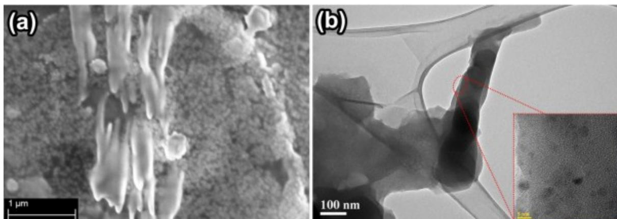
Figure S9: a) SEM image of the solution after 60 minutes of ablation at 2.4W. Some tubular structures are observable within the damaged sheets; b) TEM and HRTEM (inset) images of the tubular structures. These structures are made up of folded sheets where some GQDs are found to be embedded in.
