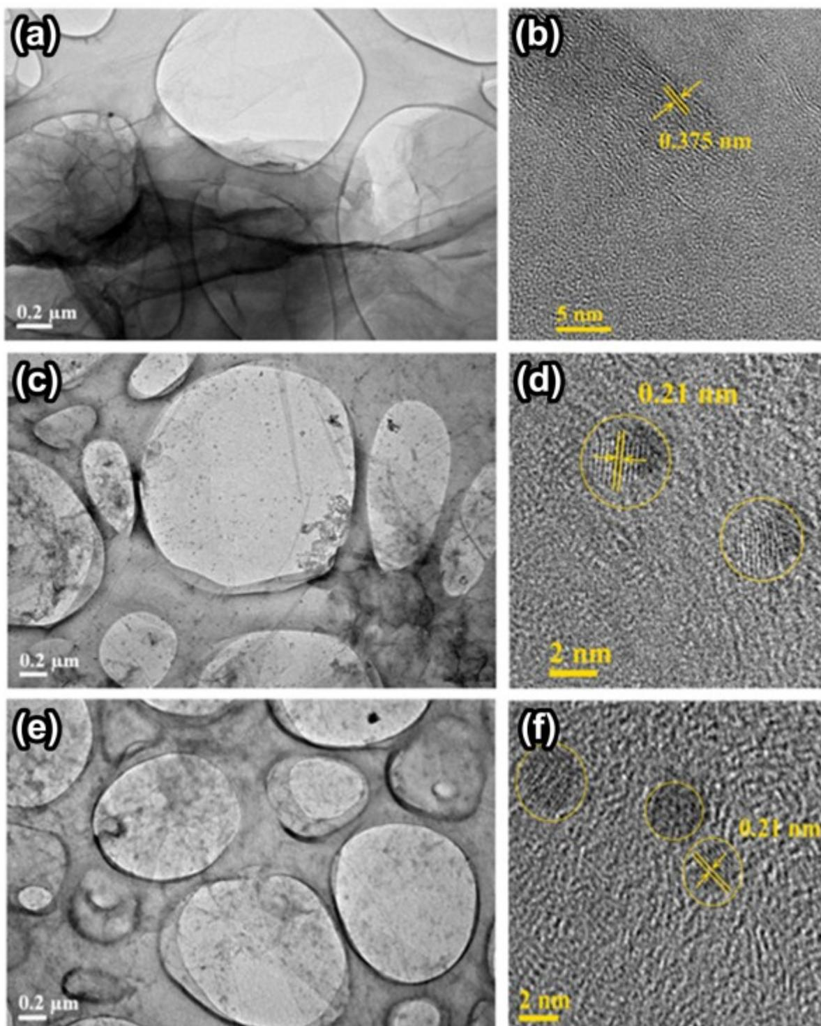
Figure S3: TEM images of a) non-treated GO solution and GO solution after (c) 5, (e) 15 minutes of laser ablation. In panel (b) HRTEM image of the non-modified GO sheets shows an interlayer d-spacing of 0.375 nm, which is larger than that of the graphite due to the presence of oxygen/containing groups. HR images (d) and (f), show the presence of few graphene quantum dots within the graphene oxide sheets after 5 and 15 minutes of laser treatment, respectively.
