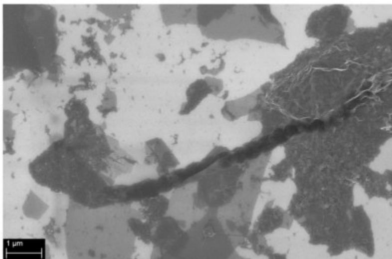
**Figure S1: SEM image of GO sheets after 5min of laser ablation. It should be noted that some layers appear twisted and we hypothesize that it might be due to the stirring of the solution**
