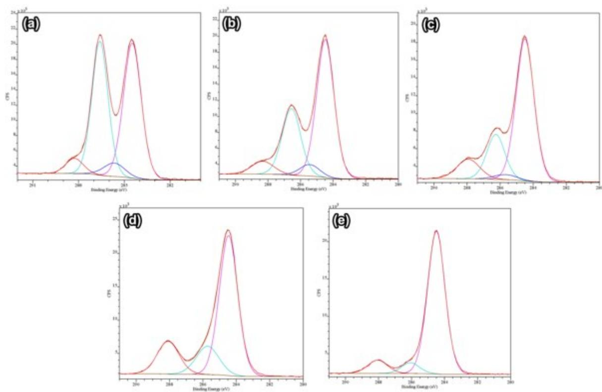
**Figure S6: XPS of GO solution before (a) and after PLA at 1.3W for (b) 5, (c) 15, (d) 30 and (e) 60 minutes respectively.**
