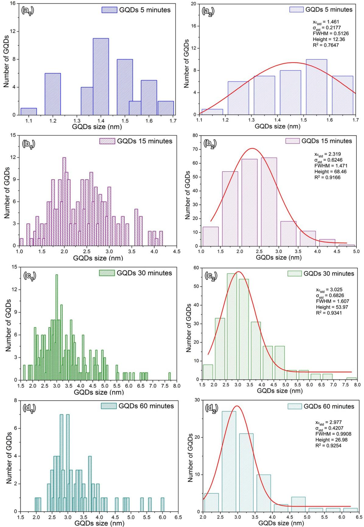
Figure S7: (1) Raw and (2) binned size distribution Size distribution of the GQDs obtained at 2.4W after (a) 5, (b) 15, (c) 30, and (d) 60 minutes of laser ablation
