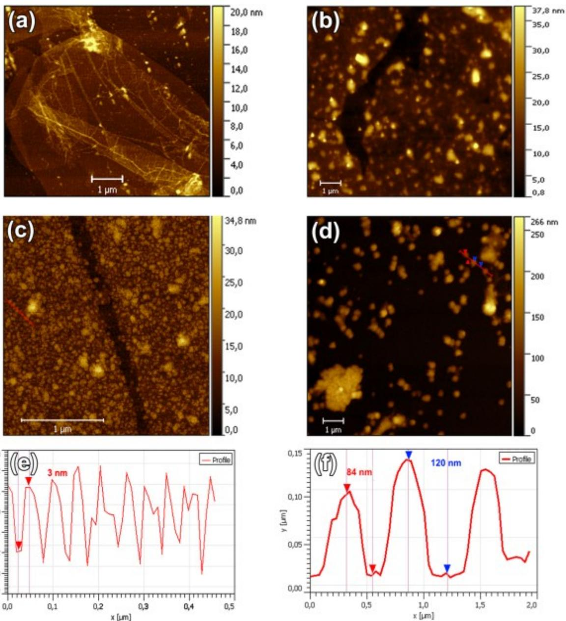
Figure S2: AFM images of the GO dispersions after (a) 5 minutes, (b) 15 minutes, (c) 30 minutes and (d) 60 minutes of laser ablation; (e) and (f) height profiles of image (c) and (d) respectively.
