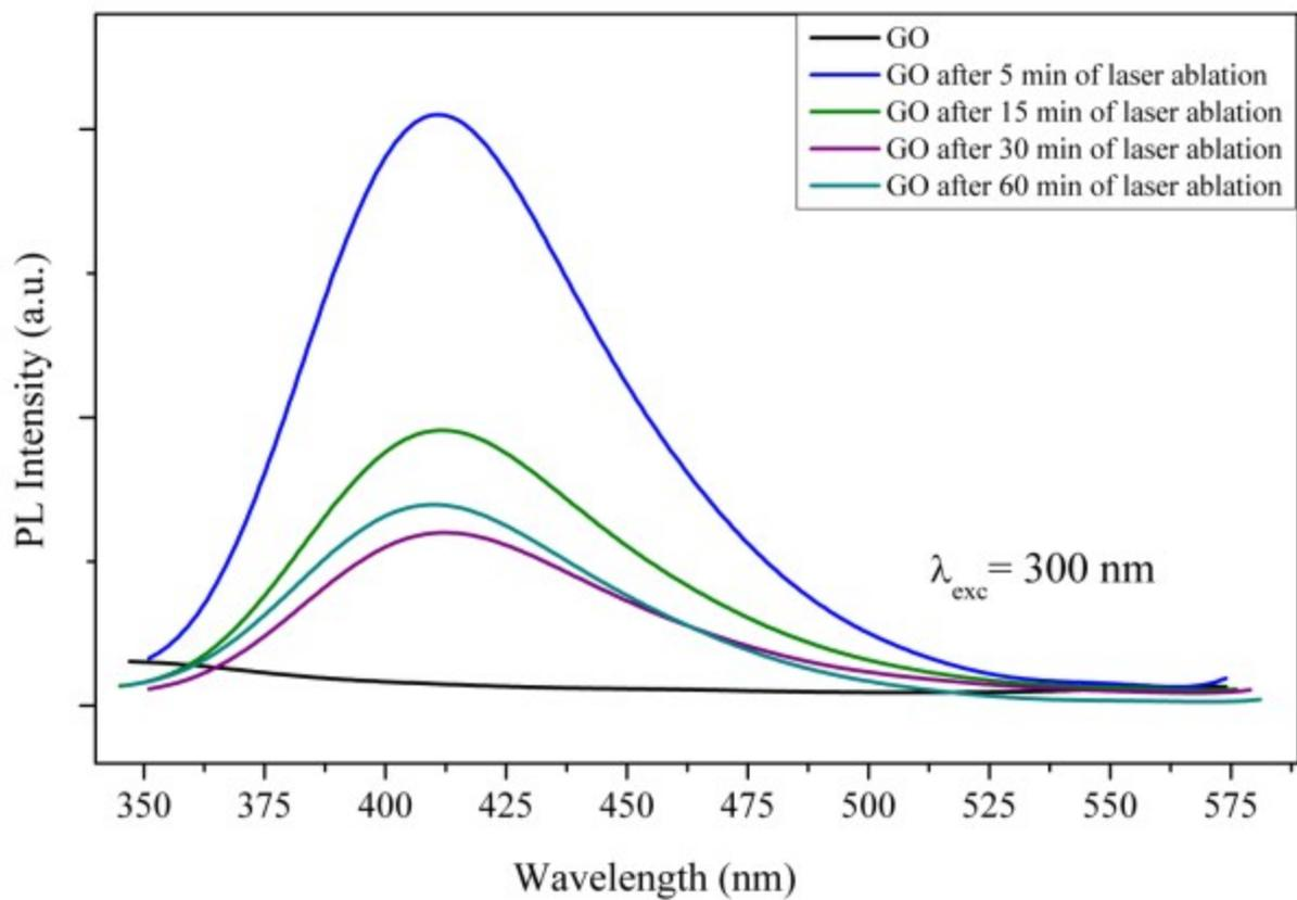
Figure S10: PL spectra of GQDs solutions obtained after 5, 15, 30 and 60 minutes of laser ablation of GO. The PL spectra were recorded at an excitation wavelength of 300 nm. The laser treated solutions showed blue luminescence at 410 nm, while the starting GO did not show any luminescence.
