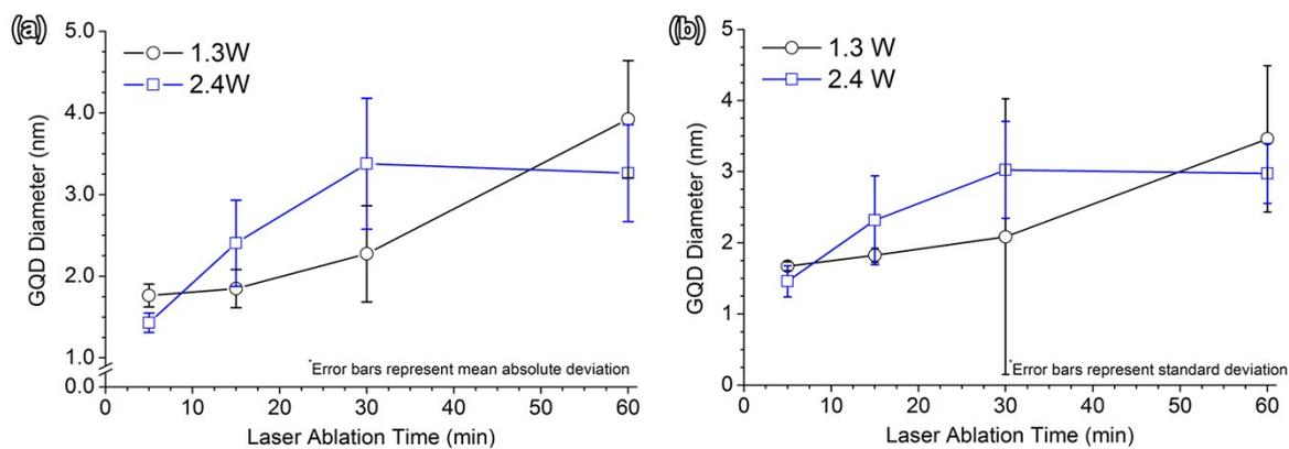
**Figure S8: GQDs diameter as a function of the laser ablation time at different laser ablation powers using (a) absolute values and (b) Gaussian fit values from binned size distribution.**
