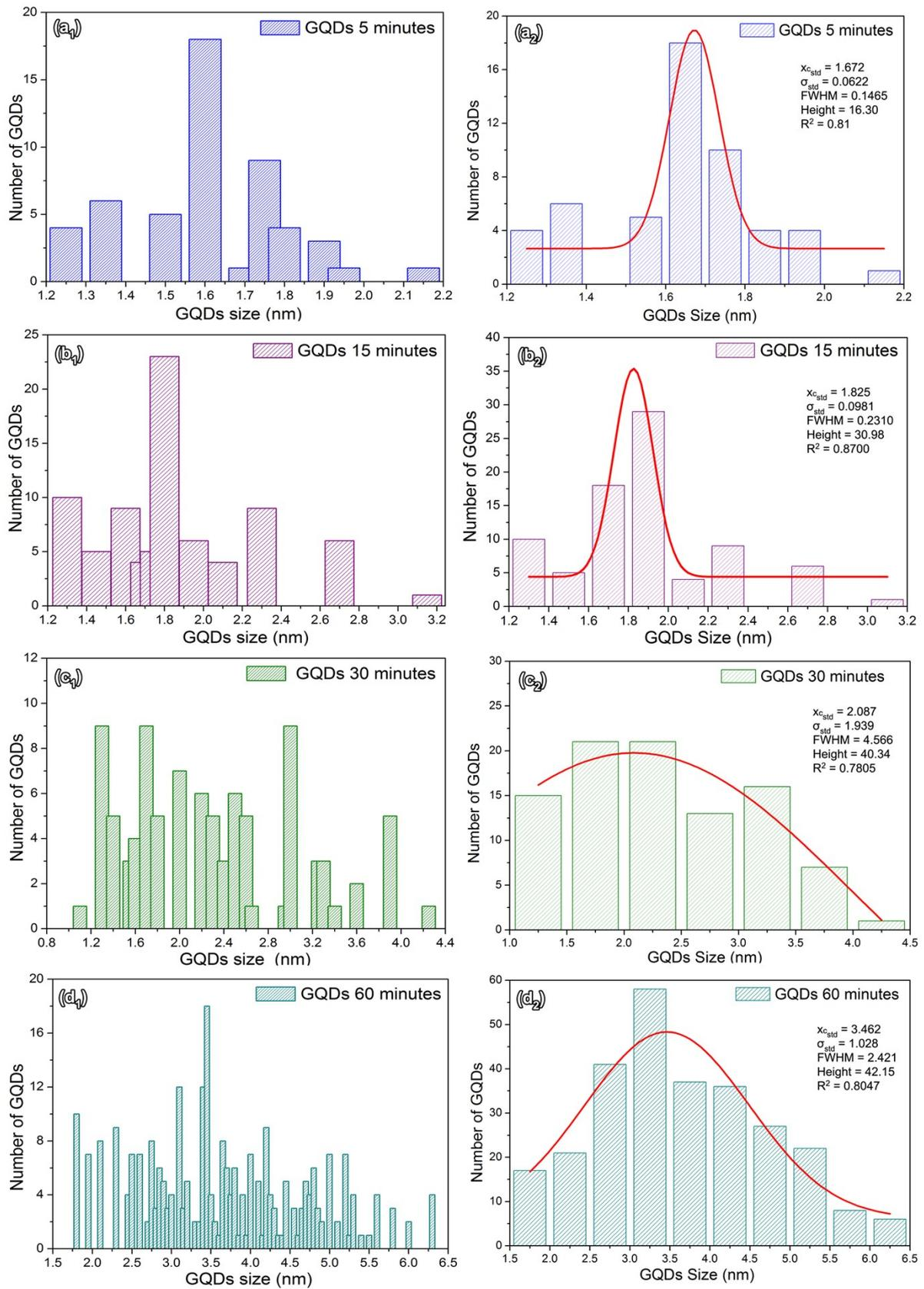
Figure S4: (1) Raw and (2) binned size distribution of GQDs after (a) 5 minutes, (b) 15 minutes, (c) 30 minutes and (d) 60 minutes of laser ablation at 1.3W
