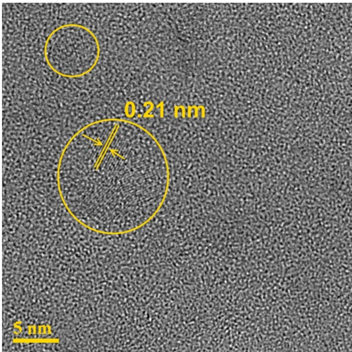
Figure S5: HRTEM image of dialysed GQDs dispersion obtained after 30 minutes of laser ablation.
