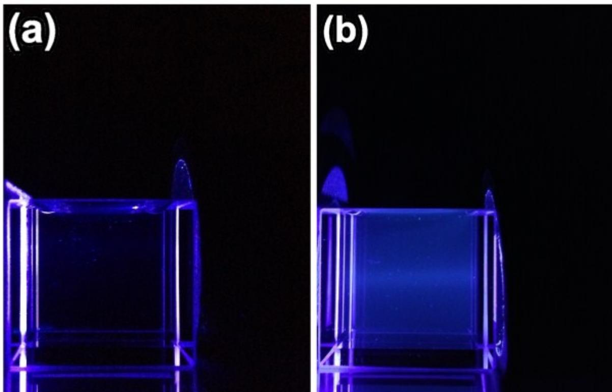
**Figure S11: Photographs of (a) water and (b) dialysed GQDs dispersion obtained after 30 minutes of laser ablation at 1.3W under 365 nm UV light.**
