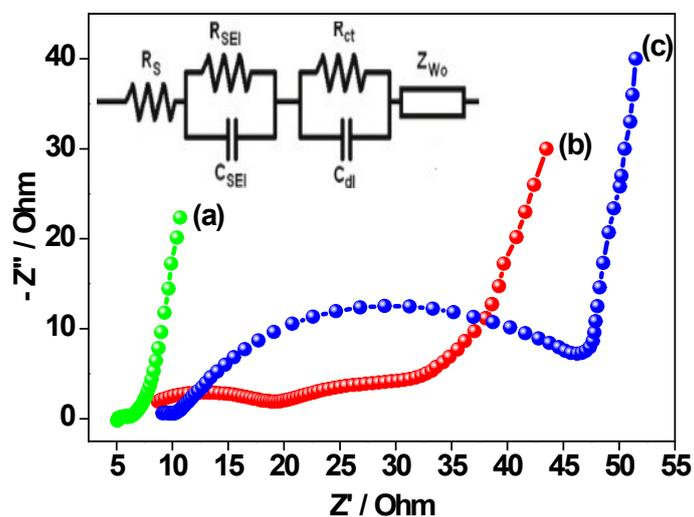
**Figure S3** Nyquist plots for the asymmetric capacitor  $\text{AC}|\text{NaNiPO}_4$  obtained by the electrochemical impedance spectroscopy. The  $\text{NaNiPO}_4$  electrodes synthesized at 300 °C, 400 and 550 °C are shown in (a), (b) and (c) respectively. The inset shows the equivalent circuit.
