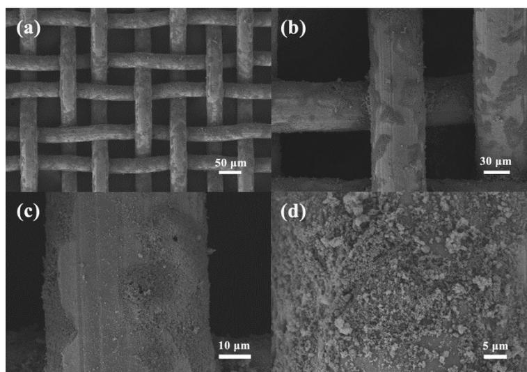
**Fig. S1** FE-SEM images of the pure hydrophobic SiO<sub>2</sub> coated mesh.
