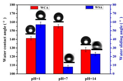
**Fig. S3** Variation of water CAs and SAs of the pure silica coated mesh with the change of pH value.
