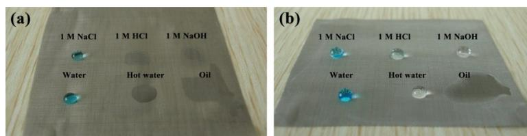
**Fig. S6** Photographs of 1M NaCl, 1M HCl, 1M NaOH solutions, hot water and kerosene droplets placed on the original (a) and (b) pure silica coated mesh.
