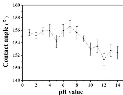
**Fig. S2** Variation of water CAs of the overlap coated meshes as a function of pH value.
