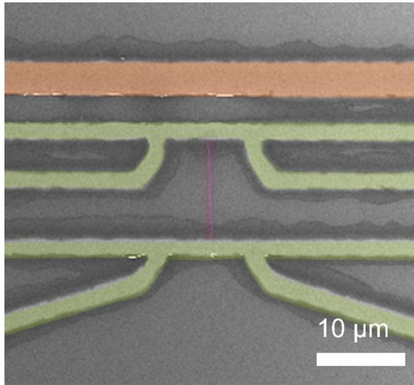
S3. SEM image of the microdevice used for thermoelectric measurement. The heating line (light orange) generates a temperature gradient along the NW, and two pairs of 4-point thermometer (light green) read the temperature difference at the hot and cold end of the NW from their resistance change. The Seebeck voltage is measured as the voltage difference between the hot and cold end.
