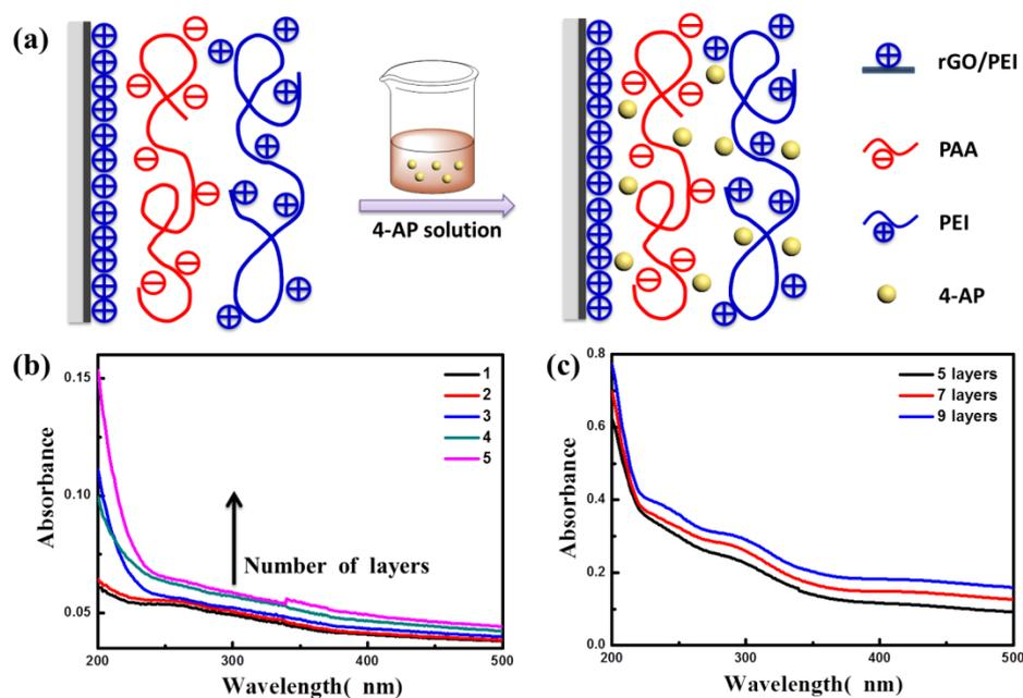
**Figure S9.** (a) Illustrative experimental setup for the penetration nature of the polyelectrolyte multilayers to 4-AP, UV-vis spectra of (b) process of the rGO/(PEI/PAA)<sub>n</sub>/PEI thin film on the quartz plates and (c) the permeability of 4-AP with different layers.
