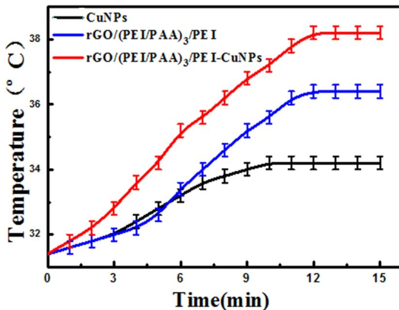
**Figure S6.** Photothermal performance of CuNPs prepared using sodium borohydride as the reducing and protecting agents, rGO/(PEI/PAA)<sub>3</sub>/PEI complex and rGO/(PEI/PAA)<sub>3</sub>/PEI-CuNPs complex.
