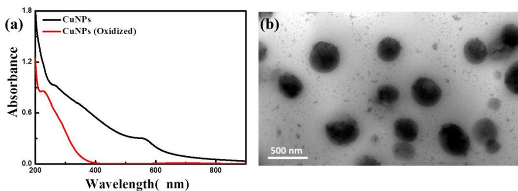
**Figure S4.** (a) UV-vis spectra of the CuNPs (black) synthesized using sodium borohydride as the reducing reagent and the CuNPs (red) kept overnight in ambient conditions. The spectra indicated that upon keeping overnight, the CuNPs were partially oxidized. (b) TEM image of (partially oxidized) CuNPs.
