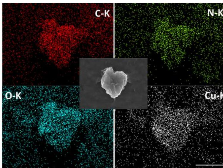
**Figure S2.** Elemental mapping of rGO/(PEI/PAA)<sub>3</sub>/PEI-CuNPs complex. The scale bars in the images corresponded to 10 μm.
