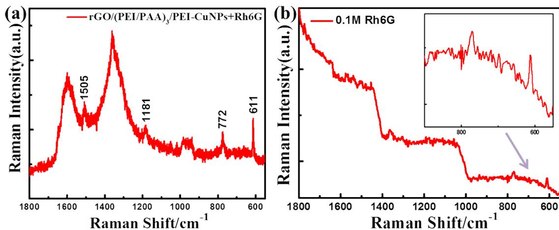
Figure S8. (a) SERS of Rh6G on the substrate of rGO/(PEI/PAA)<sub>3</sub>/PEI-CuNPs composite particles. (b) Regular Raman spectra of the Rh6G solution (0.1 M).
