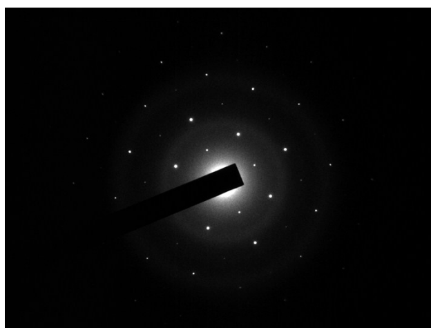
Figure S6. The SAED pattern of one FeS 2 nanosheet, which presents the single-crystalline feature.
