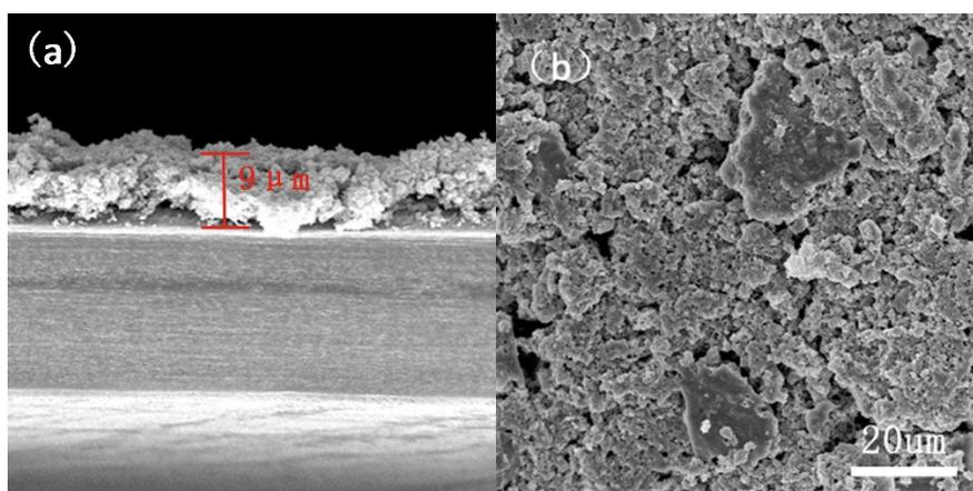
**Figure S5.** (a) Section view and (b) front view of the membrane modified by and HPC@SnO<sub>2</sub>
