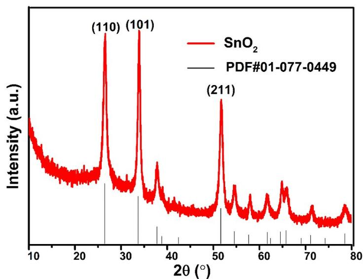
Figure S1. XRD pattern of ethanol-thermal method synthesized pure SnO<sub>2</sub>
