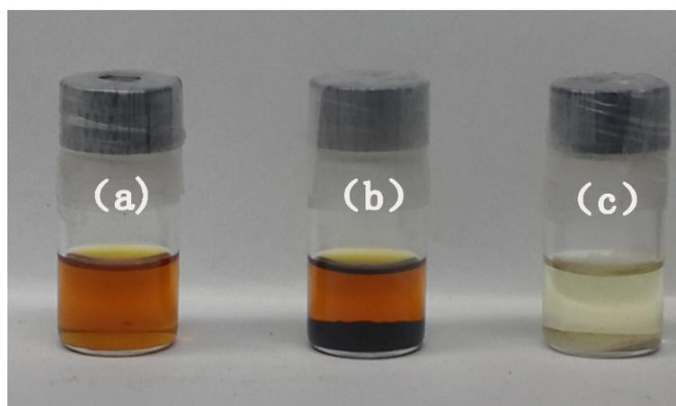
Figure S3. A visualized experiment to exhibit the adsorption ability of SnO<sub>2</sub>. (a), pristine Li<sub>2</sub>S<sub>4</sub> solution; (b), the solution with Super P; (c), the solution with SnO<sub>2</sub>.
