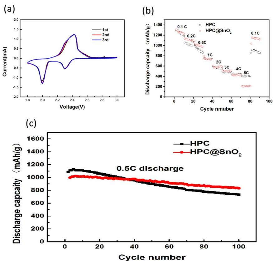
**Figure S7.** The electrochemical performance of HPC and HPC@SnO<sub>2</sub> modified membrane: (a), CV curve of HPC@SnO<sub>2</sub> modified membrane; (b), rate performance of HPC and HPC@SnO<sub>2</sub> modified membrane; (c), cycle performance of HPC-modified membrane and HPC@SnO<sub>2</sub>-modified membrane at 0.5 C.
