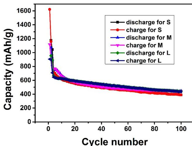
**Figure S4.** Cycle performance of coin cells with different sized cathodes
