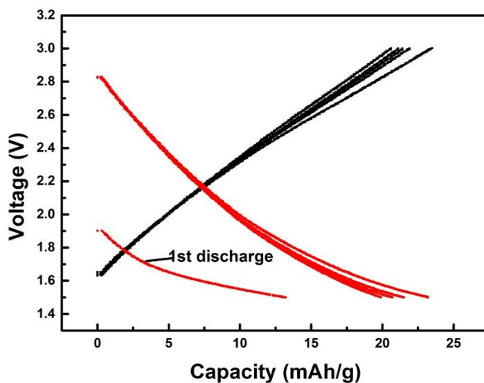
**Figure S6.** Discharge-charge profile of pure HPC@SnO<sub>2</sub> cathode at a current density of 100 mAh g<sup>-1</sup> SnO<sub>2</sub>
