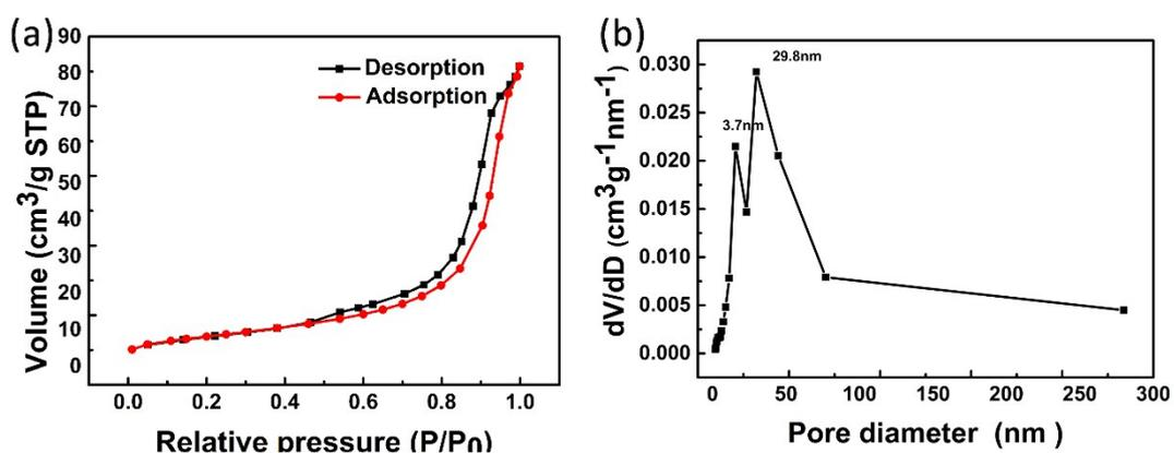
Figure S2. (a) BET isotherm curve and (b) pore size distribution of synthesized SnO<sub>2</sub>.
