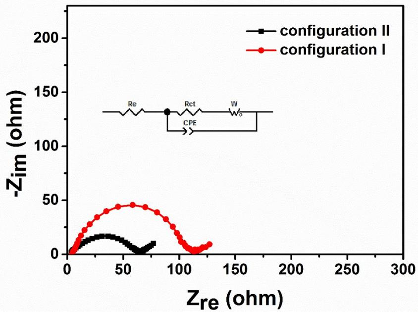
**Figure S8.** Nyquist plots for configuration II and configuration I in the frequency range of 100 mHz to 100 kHz cycling
