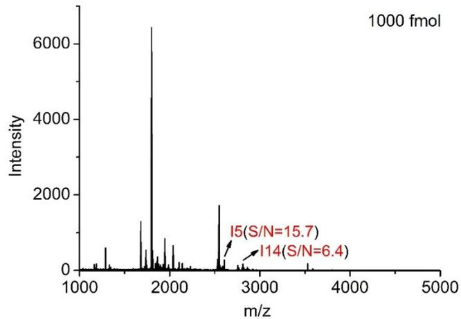
**Fig. S6** MALDI-TOF-MS spectra of IgG tryptic digest without enrichment 1000 fmol (0.5  $\mu$ L).
