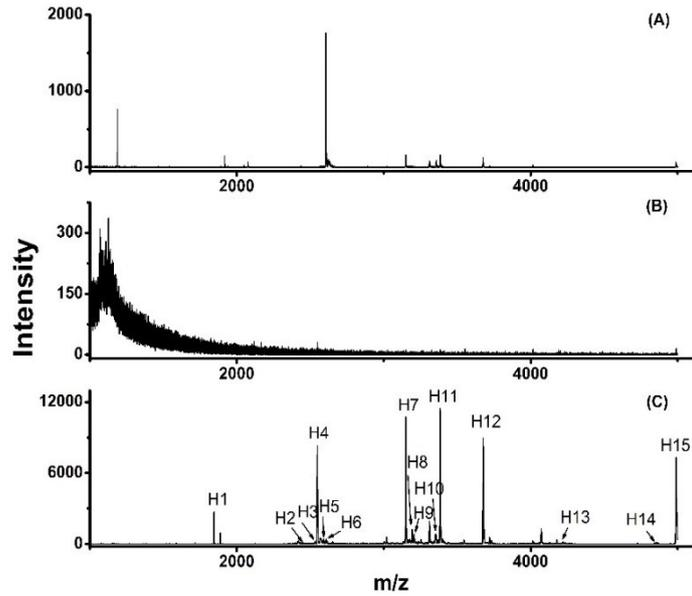
**Fig. S3** MALDI-TOF MS spectra of HRP tryptic digest (1.0 pmol/ $\mu$ L)(A) by direct analysis, (B) after MIL-101(Cr)-N<sub>3</sub> enrichment and (C) after MIL-101(Cr)-maltose enrichment.
