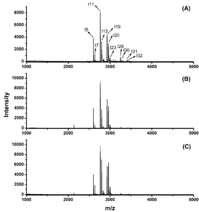
**Fig. S5** MALDI-TOF MS of glycopeptides enriched from human IgG digest (3  $\mu$ g) using MIL-101(Cr)-maltose nanoparticles, (A) for the first time, (B) for the third time and (C) for the fifth time.
