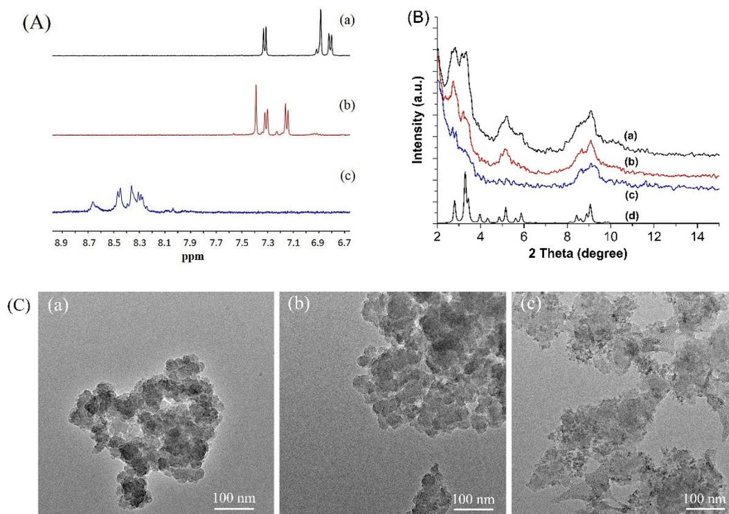
**Fig. S1** (A) <sup>1</sup>H-NMR spectra, (B) PXRD pattern and (C) TEM image of (a) MIL-101(Cr)-NH<sub>2</sub>, (b) MIL-101(Cr)-N<sub>3</sub>, (c) MIL-101(Cr)-maltose and (d) the simulated PXRD pattern calculated from MIL-101(Cr) structure.
