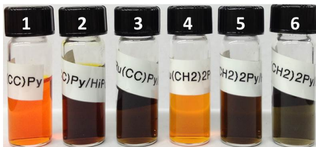
Figure S1. 1mg/ml RuPy1 and RuPy2 aqueous solutions and dispersions with SWCNTs. (1) 1mg/ml RuPy1 in water solution; (2) 1mg/ml RuPy1 with 1mg/mL HiPco SWCNTs in water solution before dialysis; (3) 1mg/ml RuPy1 and 1mg/mL HiPco SWCNTs in water solution after dialysis for 16 hours; (4) 1mg/ml RuPy2 in water solution; (5) 1
