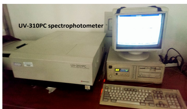
Figure S2 Photo of the measurement setup for the visible transmittance of samples.
