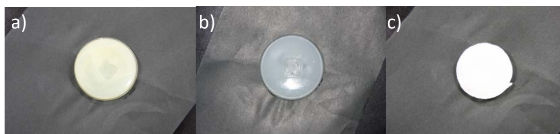
Figure S3 Photographs of free-standing gels, a) PAA porous gel, b) disordered MMT/PAA porous gel film, c) ordered layer MMT/PAA porous gel film.
