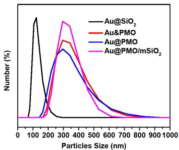
**Figure S2.** Hydrodynamic diameters of Au@SiO<sub>2</sub>, Au&PMO, Au@PMO and Au@PMO/mSiO<sub>2</sub> nanoparticles.
