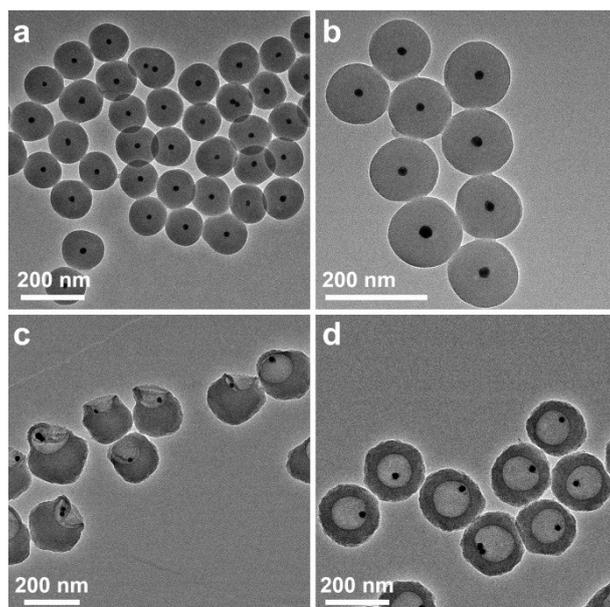
**Figure S1.** TEM images of (a), (b) core-shell Au@SiO<sub>2</sub>, (c) Janus Au&PMO, (d) yolk-shell Au@PMO nanoparticles.
