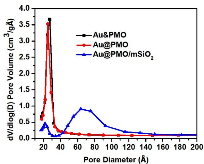
**Figure S7.** Pore size distribution curves of Au&PMO, Au@PMO and Au@PMO/mSiO<sub>2</sub> nanoparticles.
