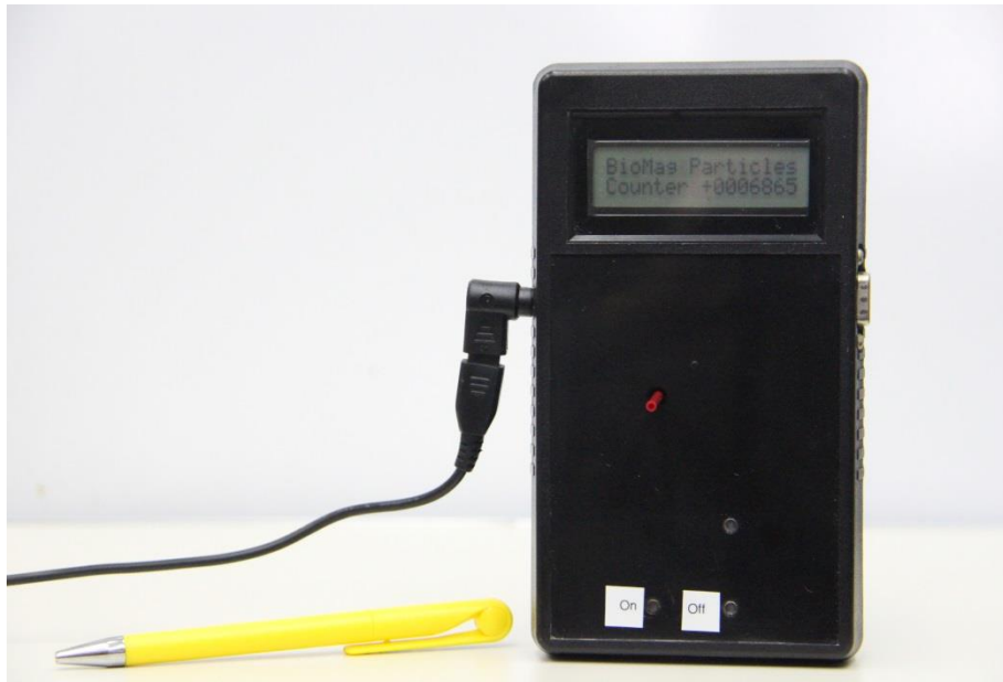
Figure S1. Photograph of the MPQ-cytometry device. Dimensions: 18 x 10 x 4 cm (H x W x D).
