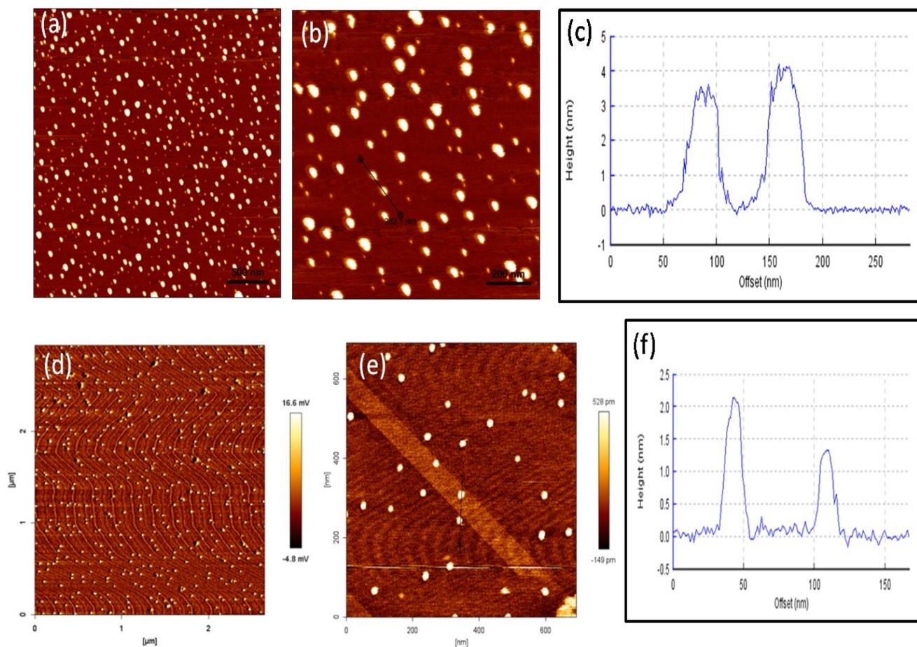
**Fig S4.** AFM images of (a, b) CTAB (10 mM) micelle<sup>2</sup>, (d, e) CTAB-QD dispersion and height profile of (c) CTAB (10 mM) micelle, (f) CTAB-QD dispersion.
