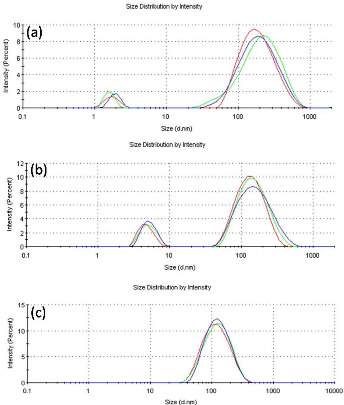
**Fig S2.** DLS measurement of (a) CTAB (10 mM) micelle, (b) cadmium chloride (10 mM) containing CTAB (10 mM) micelle and (c) CTAB-QD dispersion.
