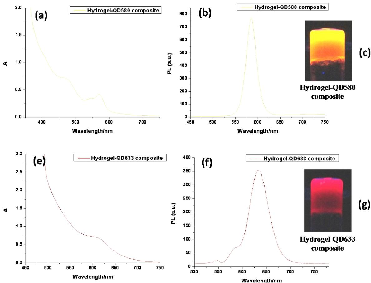
**Fig S5.** (a, e) UV, (b, f) photoluminescent spectrum and (c, g) photograph of yellow and red emitting *hydrogel-QD* composite.
