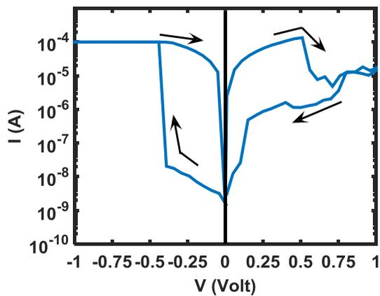
**Figure S2.** I-V curves of one switching cycle of the device measured in DI water.
