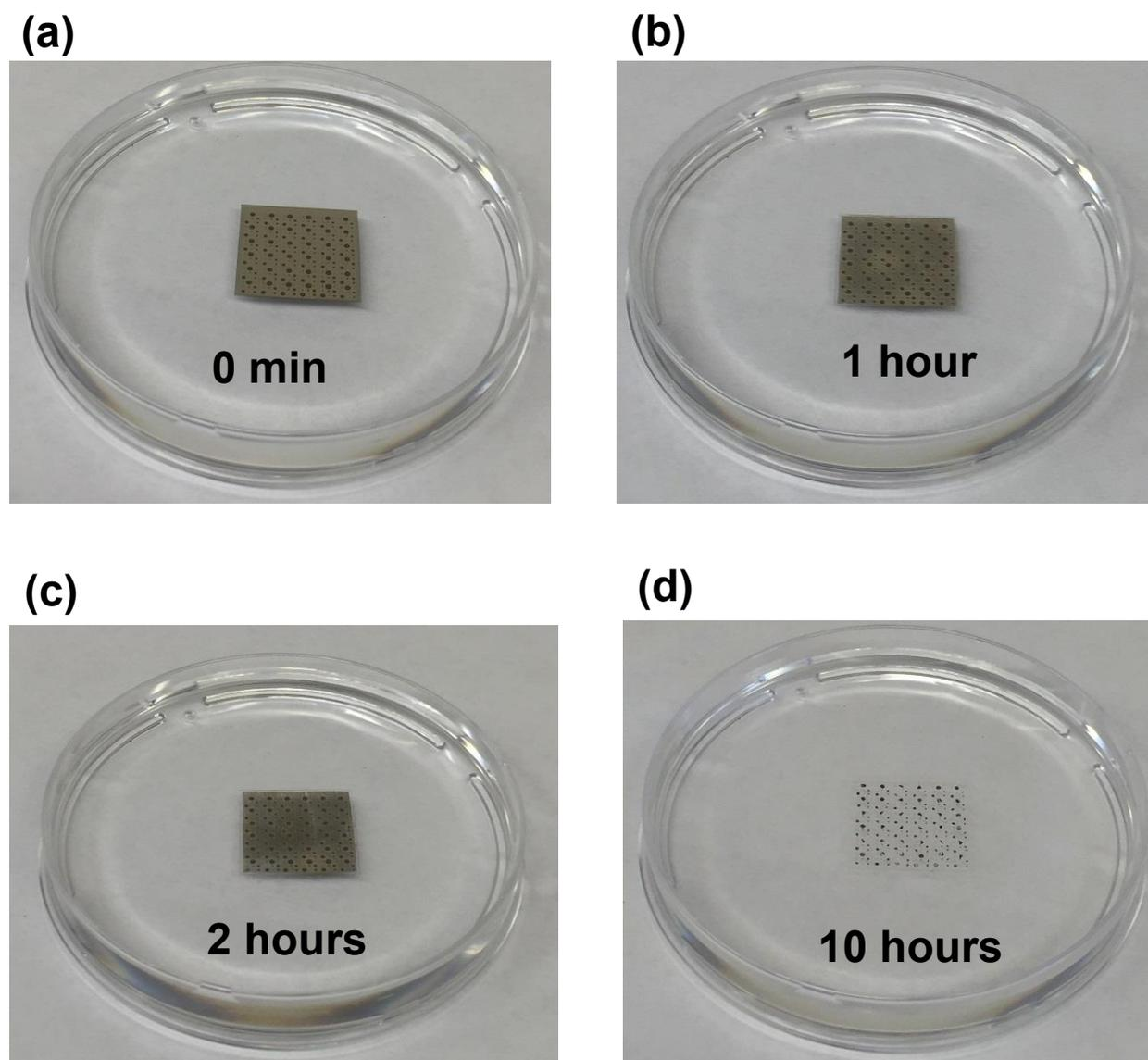
**Figure S3.** Dissolution behaviors of the PET-supported devices coated with additional 20-nm  $\text{MgF}_2$  on the front and back surfaces of the sample. Devices at (a) 0 min, (b) 1 hour, (c) 2 hours, and (d) 10 hours after immersion in DI water.
