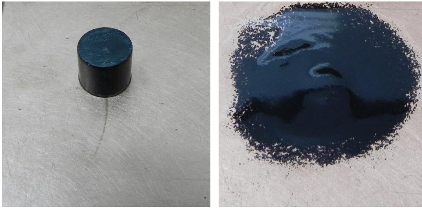
Figure S1. Simple complex of the graphene-wax mixture (i.e., no 3D foam structure of graphene) placed on a hot plate with temperature of 100°C. The weight fraction of graphene in the complex mixture was 3%. At the elevated temperature, such a complex quickly melted and collapsed, indicating its poor form stability.
