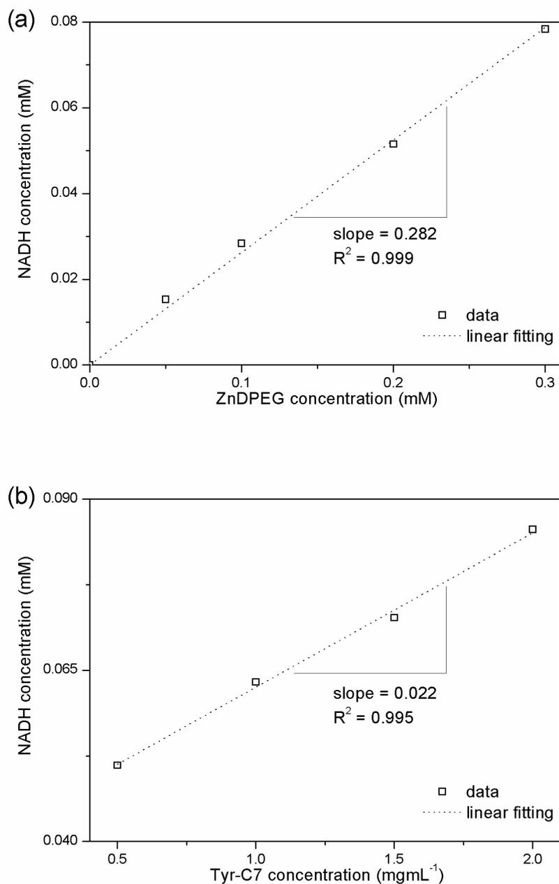
**Figure S5.** Linear dependency of NADH concentration to (a) ZnDPEG (at  $t = 15$  min) and (b) Tyr-C7 concentration (at  $t = 60$  min).
