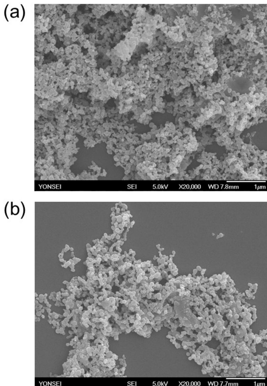
**Figure S2.** Scanning electron microscopy (SEM) images of (a) intact Tyr-C7 self-assemblies and (b) the light-harvesting systems associated with photochemical compounds.
