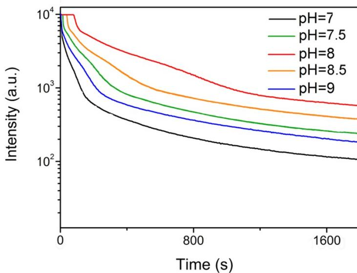
**Fig. S2** NIR afterglow decay curve of ZGGO:Cr<sup>3+</sup>,Yb<sup>3+</sup>,Er<sup>3+</sup> prepared at different pH values of starting solution. The ZGGO:Cr<sup>3+</sup>,Yb<sup>3+</sup>,Er<sup>3+</sup> was firstly irradiated with a 4 W 254 nm UV lamp for 2 min before measurement. Persistent luminescence intensity was monitored at 691 nm as a function of time (logarithmic scale).
