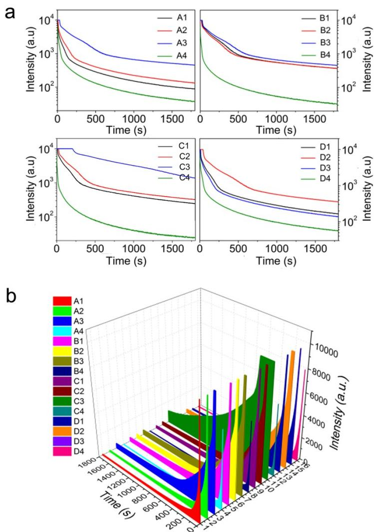
**Fig. S1** The afterglow decay curves of  $\text{Zn}_{1+x}\text{Ga}_{2-2x}\text{Ge}_x\text{O}_4:2\text{y}\%\text{Cr}^{3+}, 10\text{y}\%\text{Yb}^{3+}, \text{y}\%\text{Er}^{3+}$  powder after 5-min irradiation with a 254 nm UV lamp. (a) Two-dimensional graphs. (b) Three-dimensional graphs.
