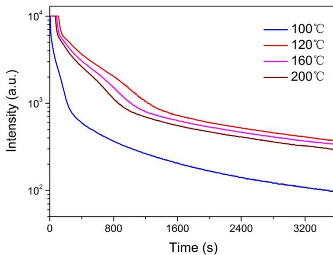
**Fig. S3** NIR afterglow decay curve of ZGGO:Cr<sup>3+</sup>,Yb<sup>3+</sup>,Er<sup>3+</sup> synthesized under different hydrothermal temperature. The ZGGO:Cr<sup>3+</sup>,Yb<sup>3+</sup>,Er<sup>3+</sup> was firstly irradiated with a 4W 254 nm UV lamp for 2 min before measurement. Persistent luminescence intensity was monitored at 691 nm as a function of time.
