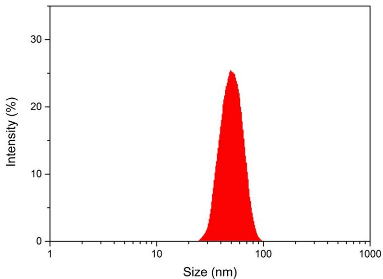
**Fig. S7** Dynamic light scattering spectra of ZGGO:Cr<sup>3+</sup>, Yb<sup>3+</sup>, Er<sup>3+</sup>.
