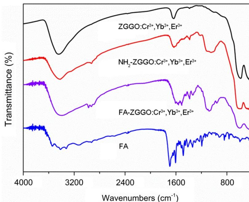
**Fig. S13** Infrared spectroscopy spectra of ZGGO:Cr<sup>3+</sup>, Yb<sup>3+</sup>, Er<sup>3+</sup>, NH<sub>2</sub>-ZGGO:Cr<sup>3+</sup>, Yb<sup>3+</sup>, Er<sup>3+</sup>, and FA-ZGGO:Cr<sup>3+</sup>, Yb<sup>3+</sup>, Er<sup>3+</sup> and folate (FA).
