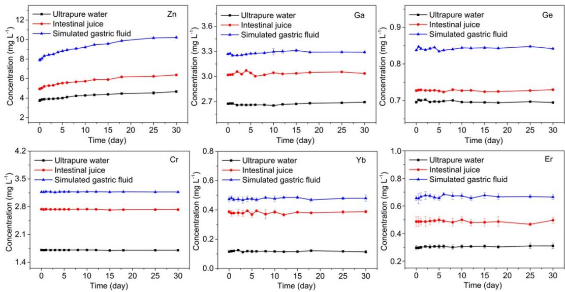
Fig. S11 Evaluation of the composition stability of ZGGO:Cr<sup>3+</sup>, Yb<sup>3+</sup>, Er<sup>3+</sup> in different media.
