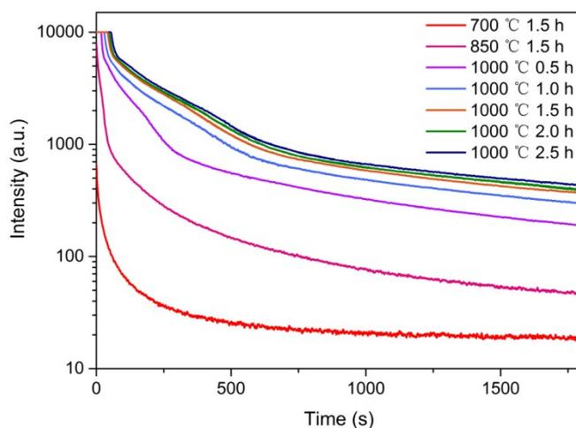
**Fig. S5** The afterglow decay curves of ZGGO:Cr<sup>3+</sup>,Yb<sup>3+</sup>,Er<sup>3+</sup> powder synthesized with different calcination time. The ZGGO:Cr<sup>3+</sup>,Yb<sup>3+</sup>,Er<sup>3+</sup> was firstly irradiated with a 4W 254 nm UV lamp for 2 min
