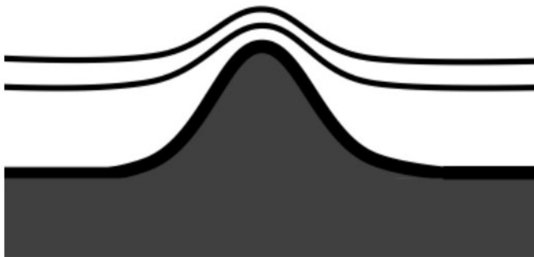
**Figure S3.** Schematic of equipotential lines around a bump.
