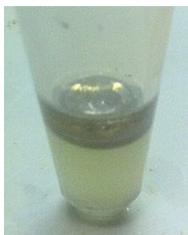
Figure S1. Photo of Ag NP monolayer at the LLI formed using the same method as for the AuNP monolayer shown in Figure 1c.
