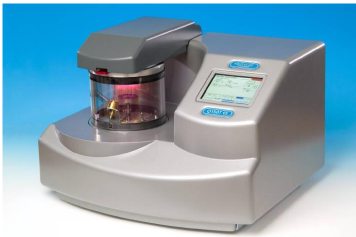
Figure S1. Quorum Q150T ES coater used for passing current through graphite.
