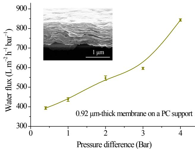
**Fig. S9** The pressure dependence of the water flux through the 0.92  $\mu\text{m}$ -thick membrane.
