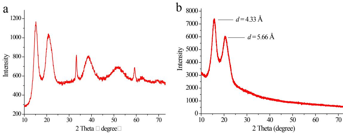
**Fig. S6** XRD spectrum of (a) the nickel hydroxide nanosheets and (b) its 3.18  $\mu\text{m}$ -thick membrane. The nanosheet sample was prepared by centrifuging the nanosheets dispersion and then dried in vacuum oven at 40 °C. The lamellar spacing ( $d$ ) was estimated on the base of the Bragg's law.
