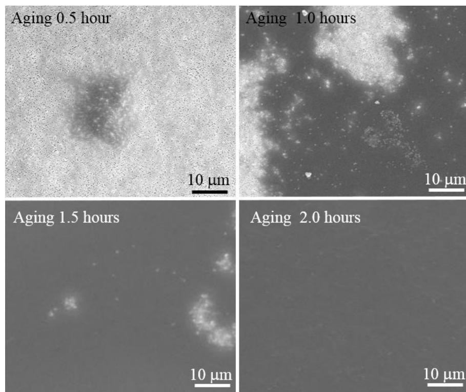
**Fig. S3** Effect of aging time on the membrane formation of the nickel hydroxide nanosheets. The membranes were fabricated by filtering the nanosheets dispersion (2.20 mL per cm<sup>2</sup> membrane) through the 200 nm-pore Anodisc filter.
