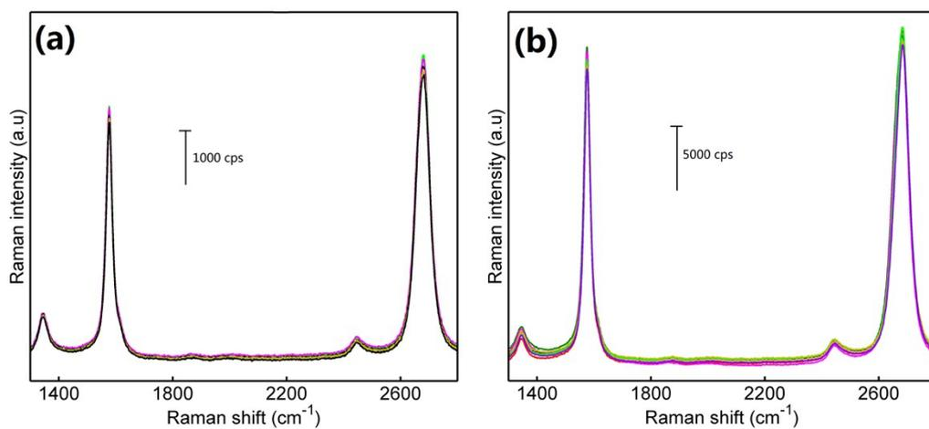
**Fig. S6** SERS spectra of monolayer graphene (a) on Ag NH arrays and (b) sandwiched between Au NPs and Ag NH arrays collected from 8 random spots.
