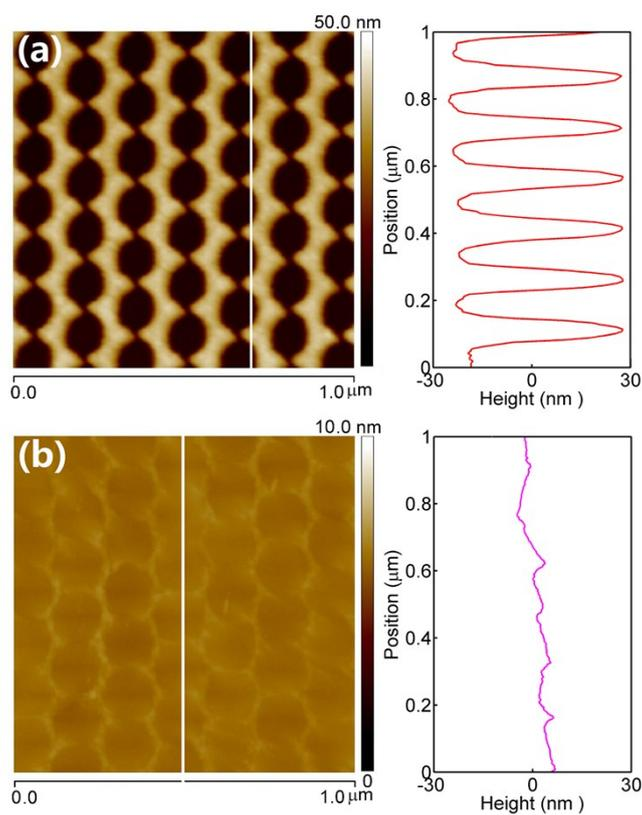
**Fig. S2** AFM images of (a) Ag NH arrays and (b) 1LG-Ag NH array structures, respectively. The right images show the cross-sections along the white lines on the left.
