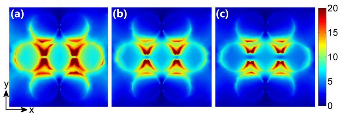
**Fig. S1** Normalized electric field intensity distributions in the xy plane for communicating Ag NH arrays with Ag tip gaps to be (a) 17 nm, (b) 36 nm and (c) 51 nm, respectively.
