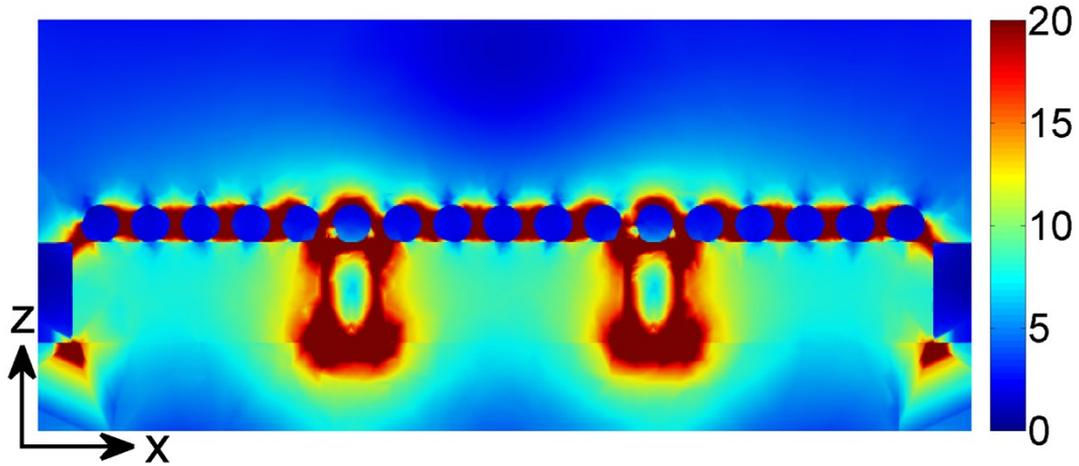
**Fig. S7** Normalized electric field intensity distribution in the xz plane for Au NP-1LG-Ag NH array structure with graphene sandwiched between Au NPs and communicating Ag NH arrays.
