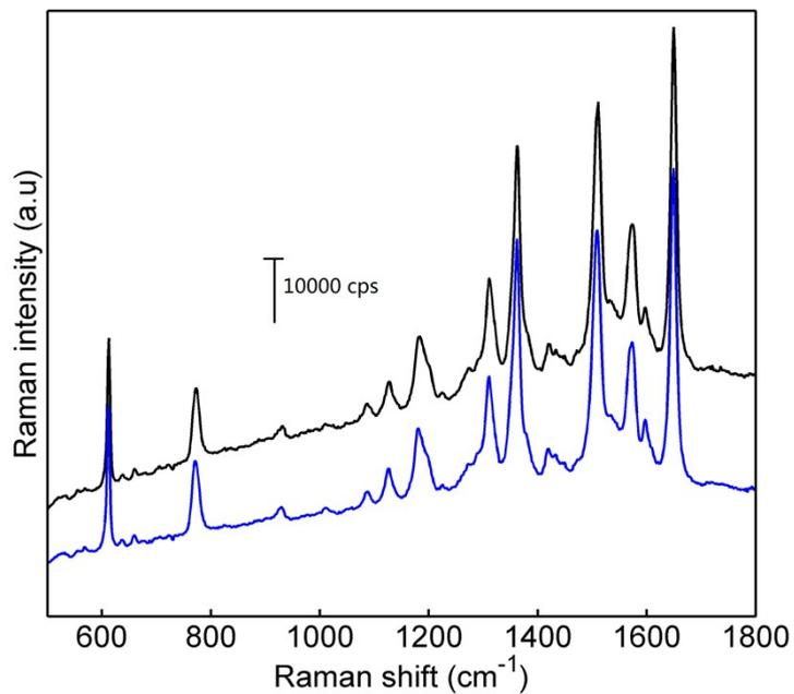
**Fig. S10** SERS spectra of  $10^{-8}$  M R6G on Au NP-1LG-Ag NH array structure measured after two days (black lines) and five months (blue lines) since the sample was prepared.
