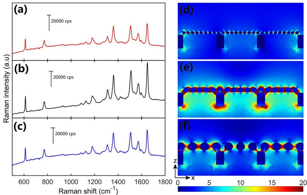
**Fig. S13** SERS spectra of  $10^{-8}$  M R6G on three different Au NP-1LG-Ag NH array structures obtained by depositing and annealing (a) 3, (b) 5, and (c) 8 nm-thick Au film on 1LG-Ag NH array structures. Normalized electric field intensity distributions of Au NP-1LG-Ag NH array structures in the xz plane at 532 nm with the diameter of Au NPs and distance between the adjacent Au NPs to be (d) 12 nm, 16 nm; (e) 20 nm, 25 nm and (f) 32 nm, 44 nm, respectively.
