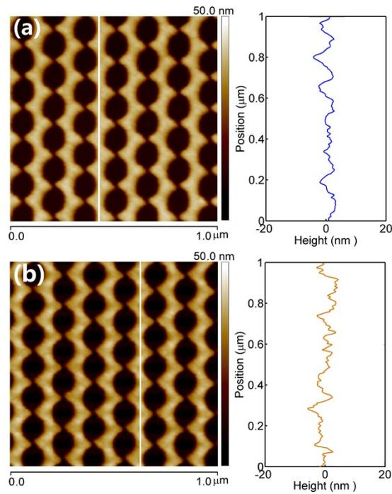
**Fig. S4** AFM images of Ag NH arrays (a) before and (b) after annealing, respectively. The right images show the cross-sections along the white lines on the left.
