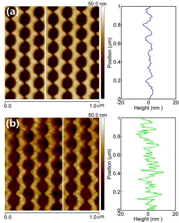
**Fig. S3** AFM images of (a) Ag NH arrays and (b) Au NP-Ag NH array structures, respectively. The right images show the cross-sections along the white lines on the left.
