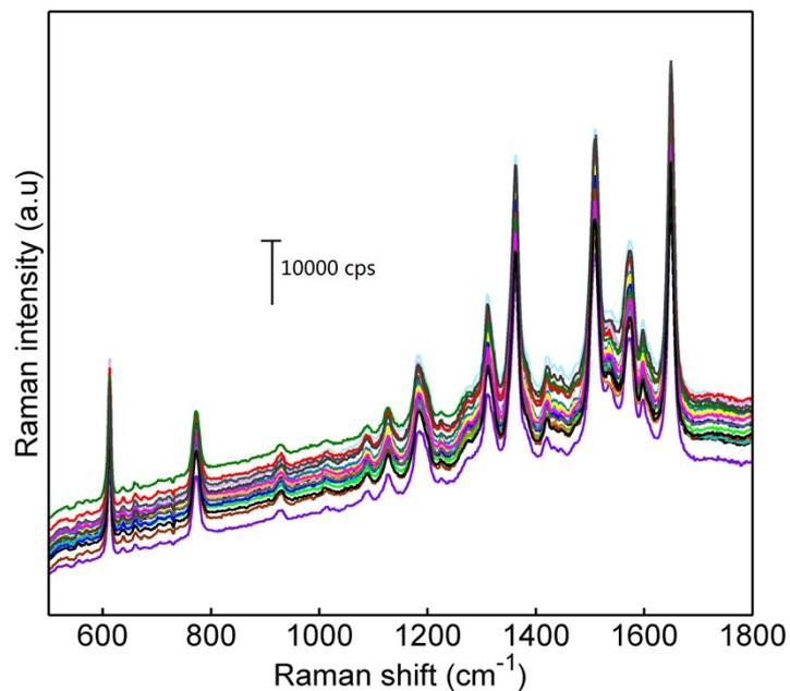
**Fig. S9** SERS spectra of  $10^{-8}$  M R6G on Au NP-1LG-Ag NH array structure collected from 20 random spots.
