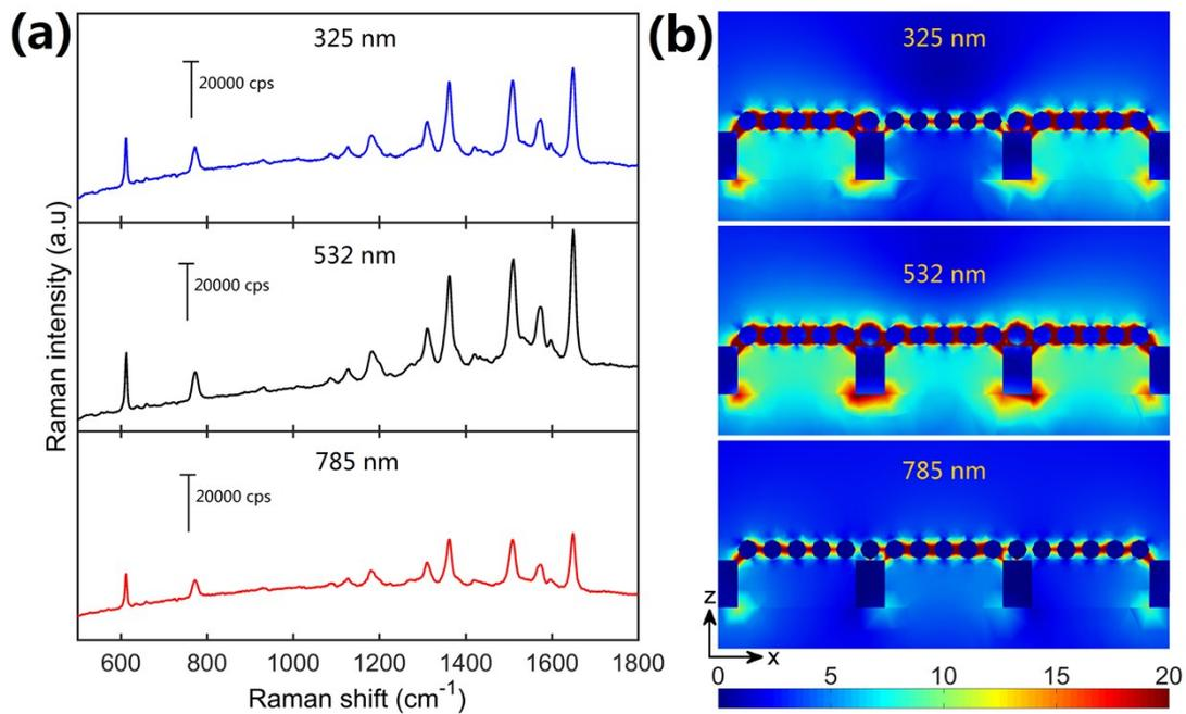
**Fig. S8** (a) SERS spectra of  $10^{-8}$  M R6G on Au NP-1LG-Ag NH array structure with excitation wavelength of 325 nm, 532 nm and 785 nm, respectively. (b) Normalized electric field intensity distributions of Au NP-1LG-Ag NH array structure in the xz plane with excitation wavelength of 325 nm, 532 nm and 785 nm, respectively.
