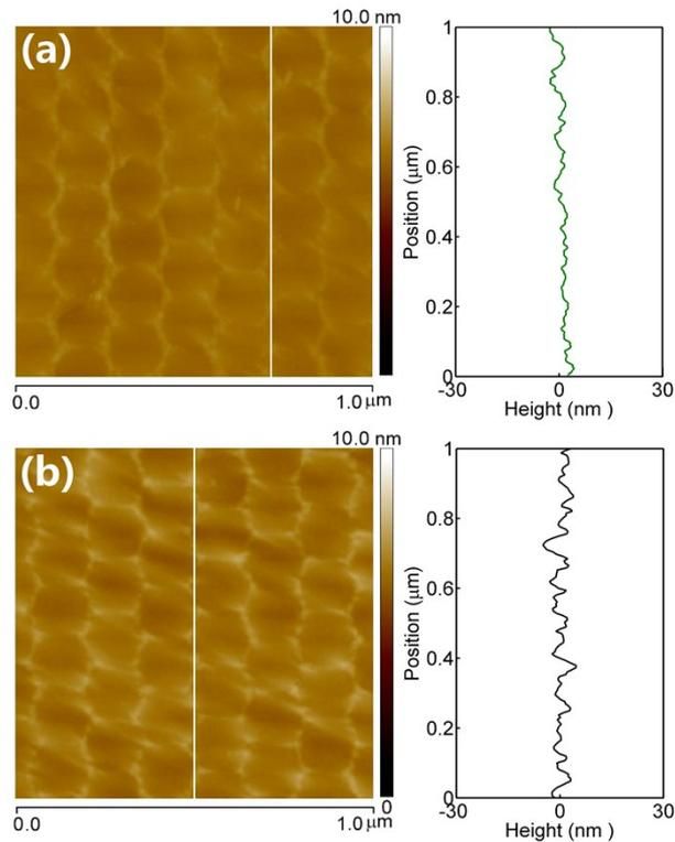
**Fig. S5** AFM images of 1LG-Ag NH array structures (a) before and (b) after annealing, respectively. The right images show the cross-sections along the white lines on the left.
