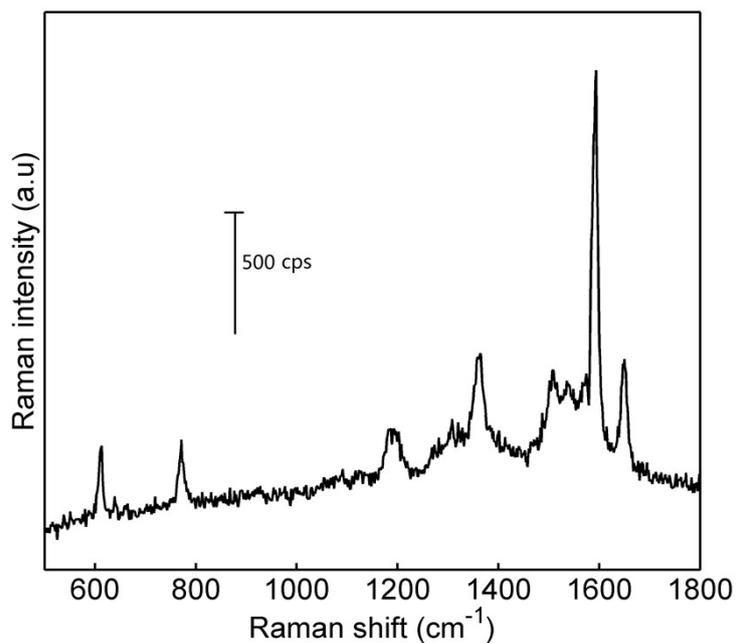
**Fig. S11** SERS spectrum of  $10^{-13}$  M R6G on Au NP-1LG-Ag NH array structure.
