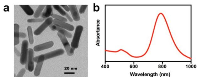
Figure S1. (a) TEM image and (b) UV-vis spectrum of GNRs.
