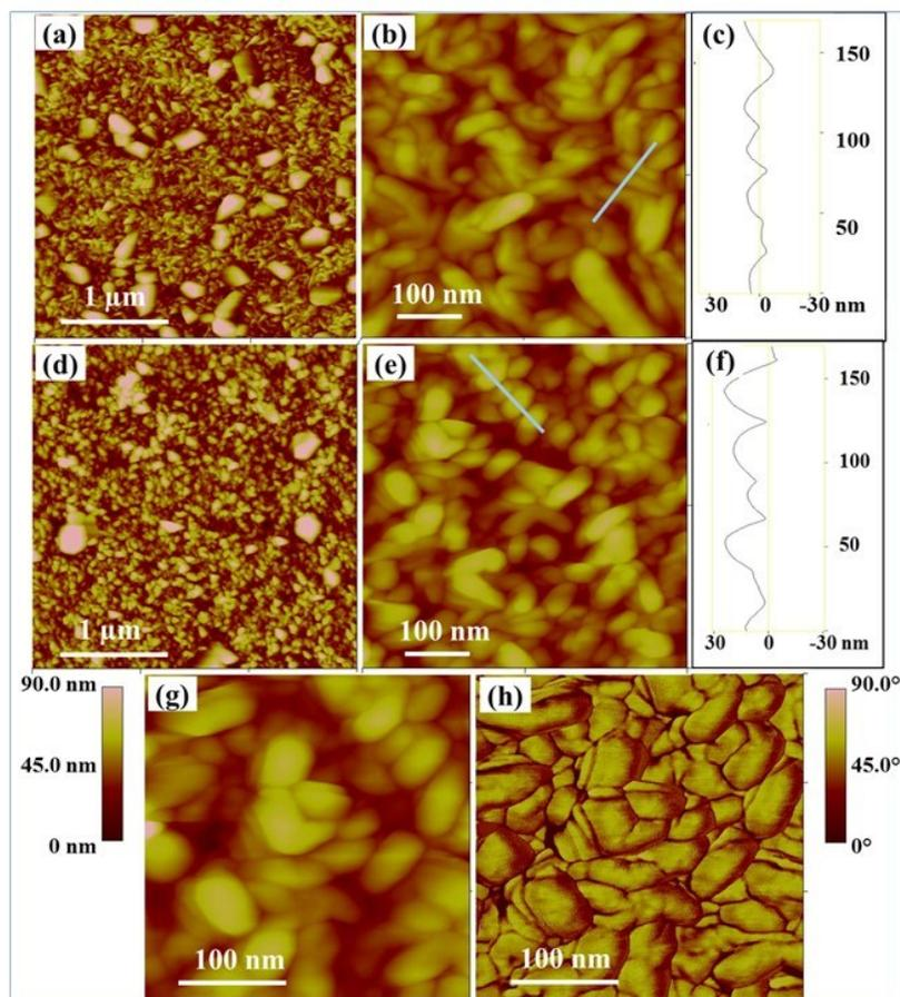
**Figure S3** Representative AFM images: a) and b) topographic images for the 300 nm S-Mo film. (d), (e) and (g) topographic images with (h) phase image of panel (g) for the 50 nm S-Mo film. In (c) and (f) the height profiles showing the typical thickness of the nanosheets from panel (b) and (e) respectively. The Z- axis scale for panels (a), (b), (d) and, (e) is the same as for (g).
