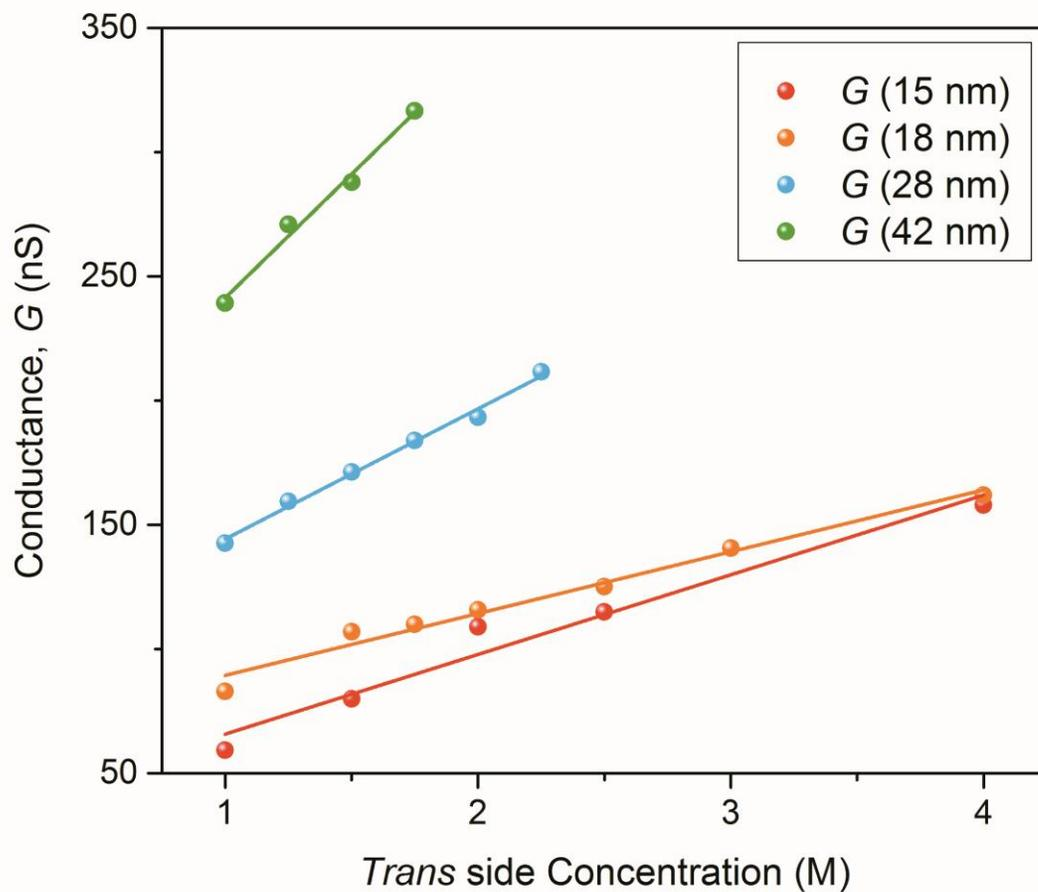
**Figure S2.** Ionic conductance of four nanopores under different electrolyte concentration gradients. The *cis* side electrolyte concentration was kept at 1 M.
