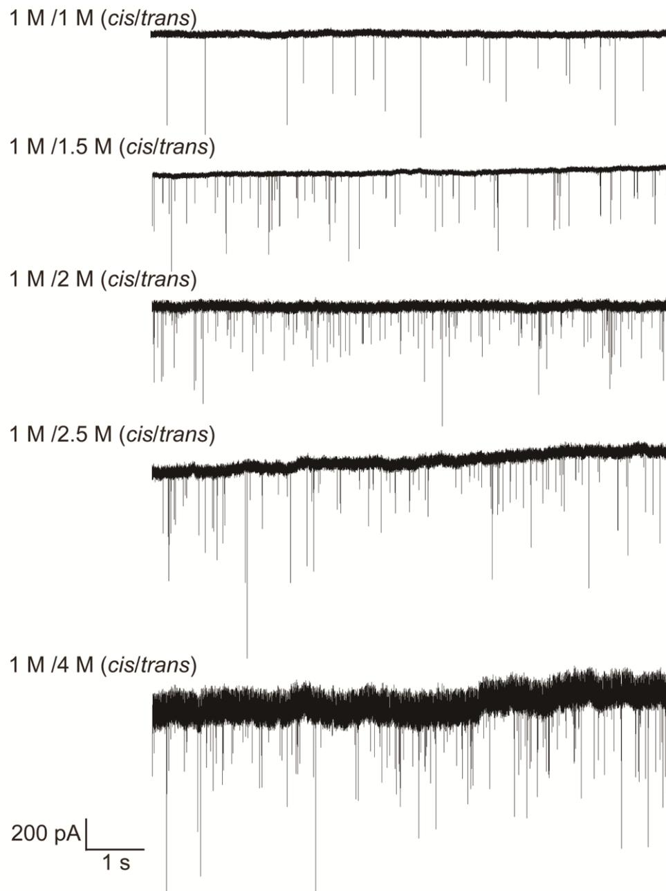
**Figure S3.** Ionic current traces with translocation of dsDNA molecules through a 15 nm nanopore with a range of concentration gradients. No positive pulse signals can be detected even when the concentration setting is 1 M/4 M (*cis/trans*).
