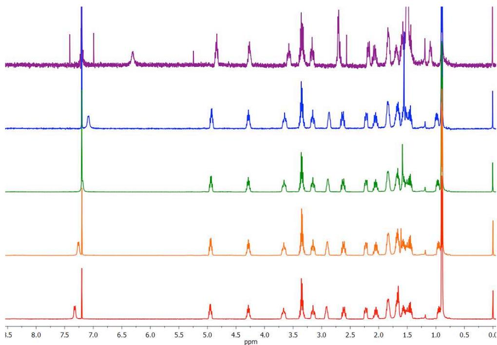
**Fig. 1SI.** Set of different  $^1\text{H}$  NMR spectra recorded for **CP1** at different concentrations (from top to bottom 1, 10, 20, 30 and 40 mM) in  $\text{CDCl}_3$  at room temperature.
