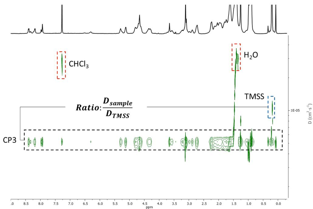
**Figure 4SI.** Representative DOSY NMR experiment of **CP3** in a 1% solution of MeOH- $\text{d}_3$  in  $\text{CDCl}_3$ , in which the different diffusion bands can be observed.
