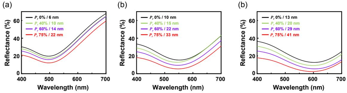
**Figure S3.** (a-c) Calculated reflectance spectra of  $P_r$  0%, 40%, 60% and 75% with different Ge thicknesses enabling the minimum dip of reflectance at each wavelength of (a) 500 nm, (b) 550 nm and (c) 600 nm.
