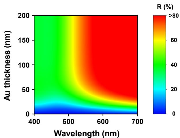
**Figure S7.** Contour plot of calculated reflectance variation as a function of Au thickness and of wavelength for determining sufficient optical thickness of Au.
