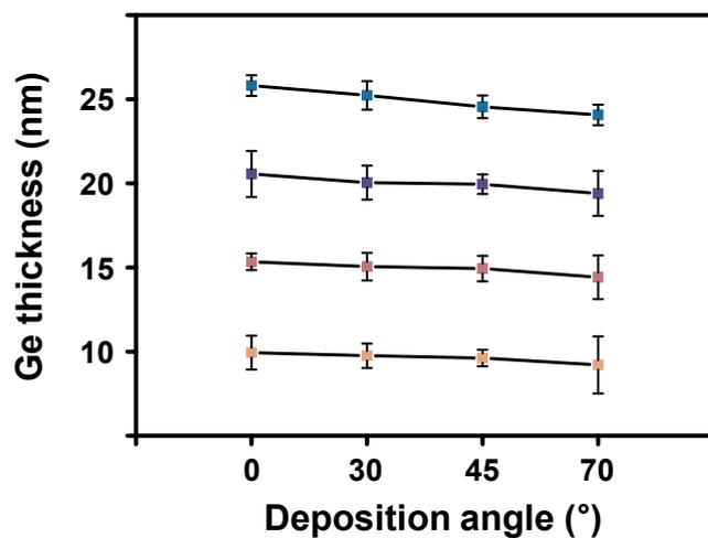
**Figure S5.** Measured Ge thickness in samples of different thicknesses (i.e. 10 nm, 15 nm, 20 nm and 25 nm) at each deposition angles (i.e. 0°, 30°, 45° and 70°) by atomic force microscopy.
