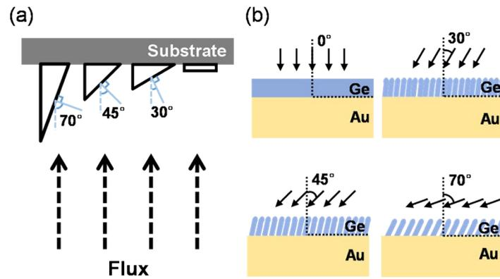
**Figure S4** (a-b) Schematic illustrations of (a) experimental setup with inclined sample holders for the oblique angle deposition of Ge films and (b) deposited Ge films on Au substrate with oblique angles of 0°, 30°, 45° and 70°
