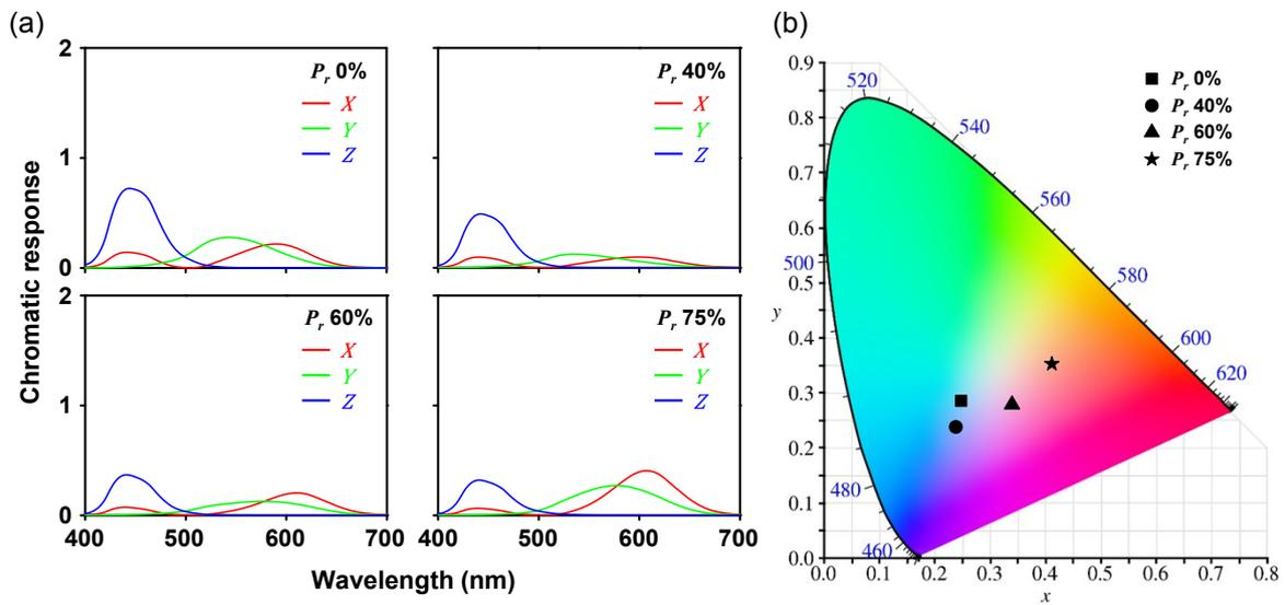
**Figure S2.** (a) Chromatic response of the tristimulus values and (b) the CIE plot with  $P_r$  0%, 40%, 60% and 75% at a Ge thickness of 20 nm.
