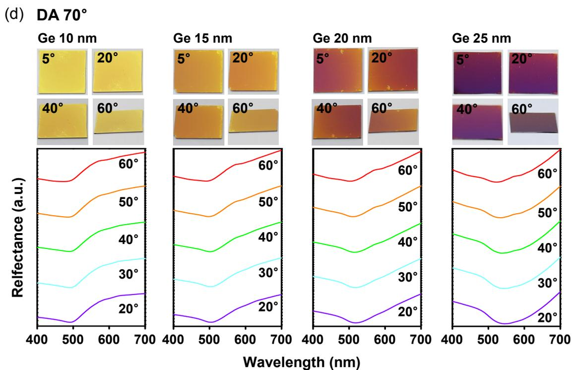
**Figure S6.** (a-d) Images with different angles of view from 5° to 60° and measured reflectance spectra at oblique angles from 20° to 60° of (a) DA 0°, (b) DA 30°, (c) DA 45° and (d) DA 70° with different thickness (i.e., 10 nm, 15 nm, 20 nm and 25 nm).
