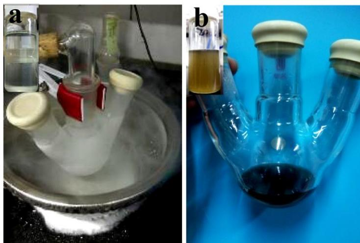
The experimental set-up diagram for metal nanoparticles preparation. (a) The two salts were freeze-dried before  $(\text{LiBH}_4)/\text{THF}$  solution adding. (b) The photograph of nanoparticles in the flask.
