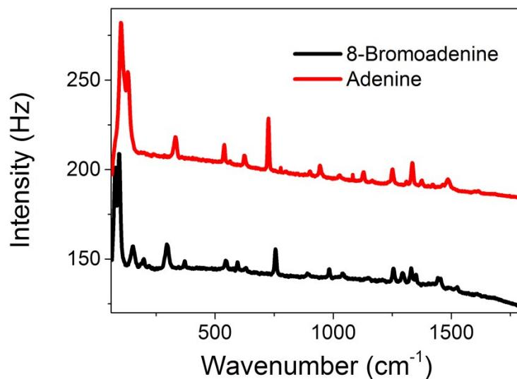
**Figure S1:** Raman spectra of <sup>8Br</sup>A and A powder taken with a 785 nm laser.
