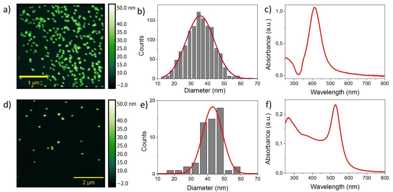
**Figure S2:** a) AFM image of AgNP, b) Size distribution of AgNP, c) UV-Vis-Absorbtion spectra of AgNP, d) AFM image of AuNP, e) Size distribution of AgNP, f) UV-Vis-Absorbtion spectra of AgNP.
